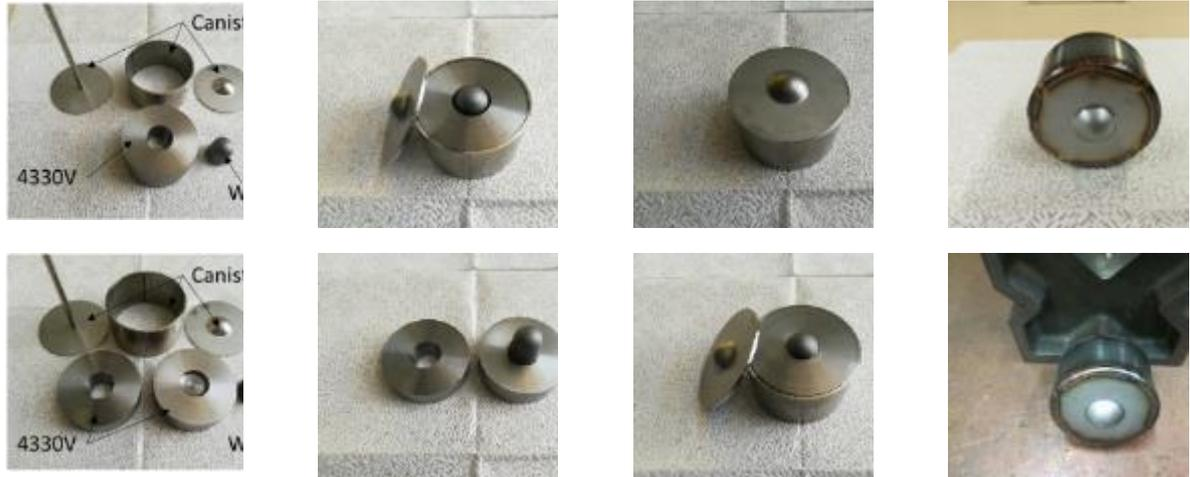
Figure 22: fabrication of the two investigated designs without metallic interlayer (reference mock-ups)
