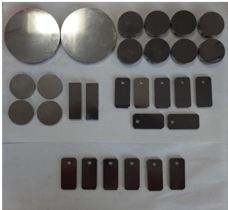
Figure 64: Photograph showing all the ENP specimens that were produced for testing in WP3
