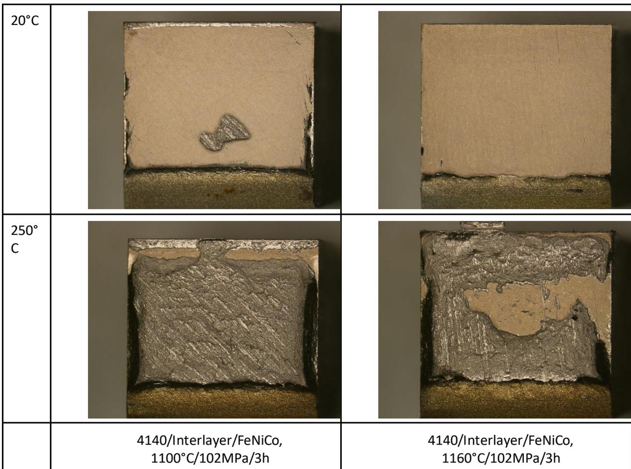
Figure 53: photographs of broken KV impact toughness specimens machined inside the 4140/interlayer N<sup>2</sup>/FeNiCo joints manufactured by HIP at 1100°C and 1160°C and tested at 20°C and 250°C.
