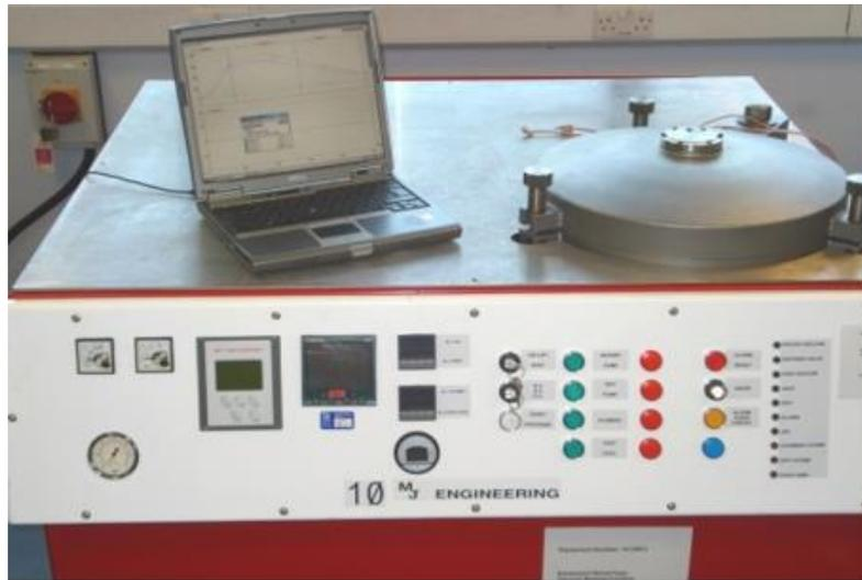
Figure 57: TWI vacuum furnace VB1
