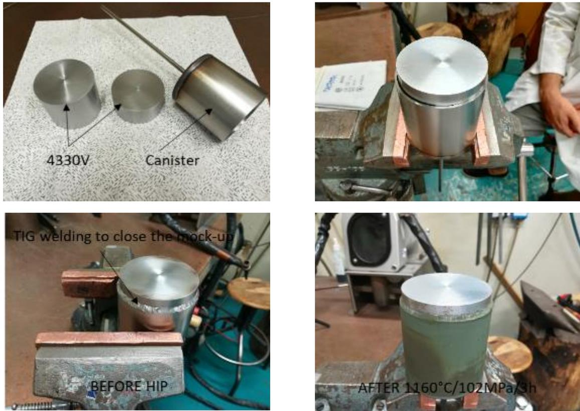
Figure 17: 4330V/4330V mock-up to evaluate the mechanical properties of the 4330V and 4330/4330V joint after a HIP done at 1160°C/102MPa/3h and post heat treatments to harden the 4330V steel to the required hardness.
