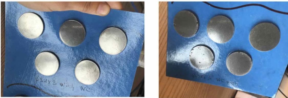
Figure 6: GO/WC fabricated pieces (left, neat WC-Co, right WC-Co + GO)
