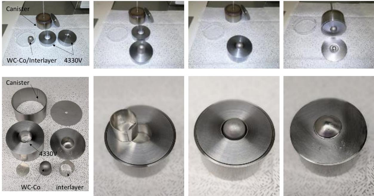
Figure 26: fabrication of the two investigated designs with the 0.1mm and the 0.5mm thick interlayers
