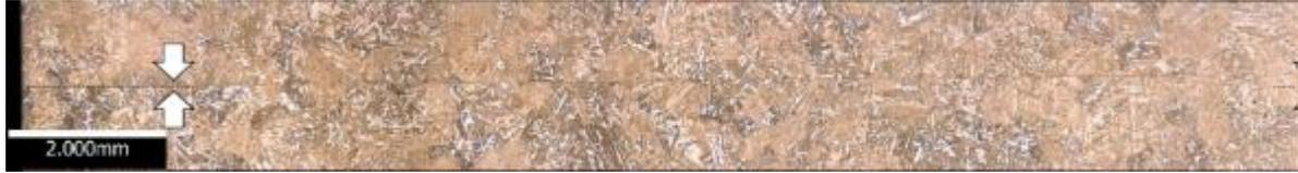
After etching with 2% Nital. The arrows indicate the localization of the joints
