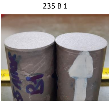
Coating adhesion failure
