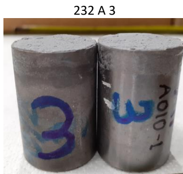
Coating cohesion failure
