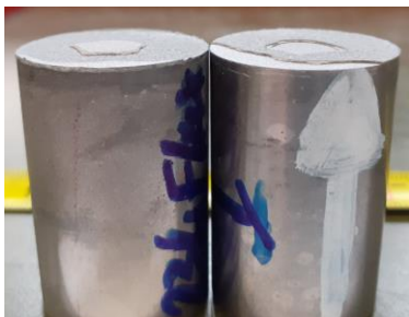
Dual failure mechanism due to both the adhesion of the coating and the failure of the glue
