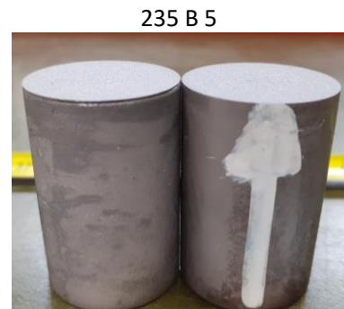
Coating adhesion failure
