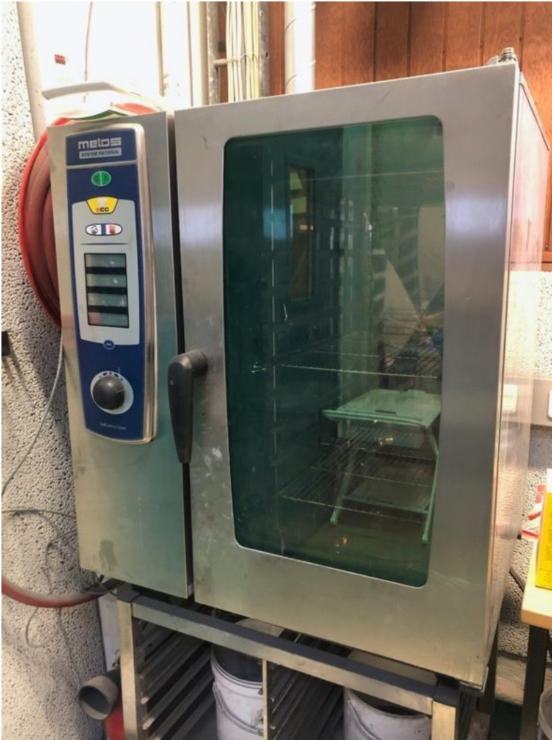
Figure 82 Oven used for lower T settings. Humidity level can be controlled.
