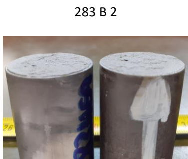
Coating cohesion failure
