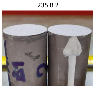
Coating adhesion failure
