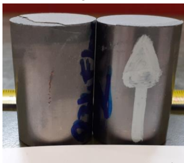
Dual failure mechanism due to both the adhesion of the coating and the failure of the glue
