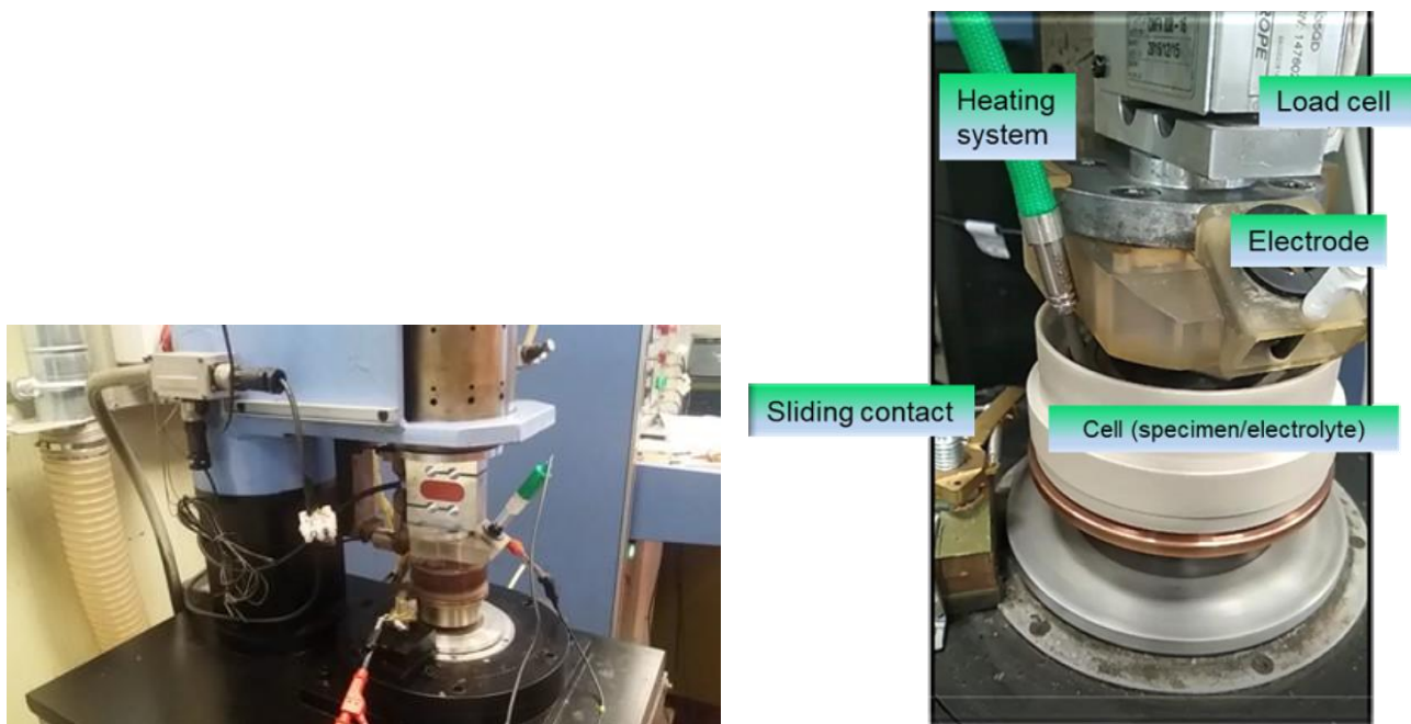
Figure 2.1.49 - The modified RTM ball-on-disk tribometer (left) with the electrochemical cell during a test. Right some details of the cell. Bottom, Xylan disk for tribocorrosion test
