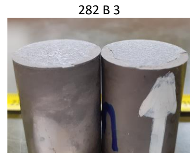
Dual failure mechanism due to both the adhesion of the coating and the failure of the glue
