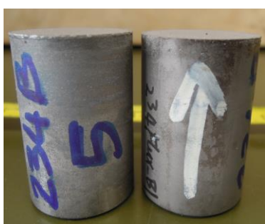
Coating adhesion failure
