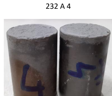
Coating cohesion failure
