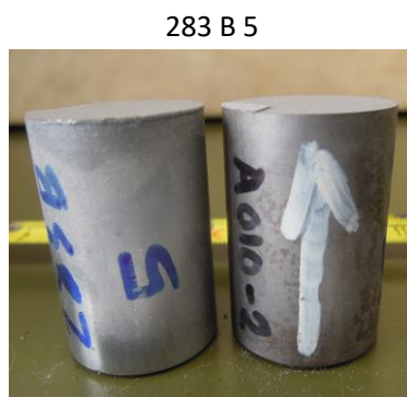
Dual failure mechanism due to both the adhesion of the coating and the failure of the glue
