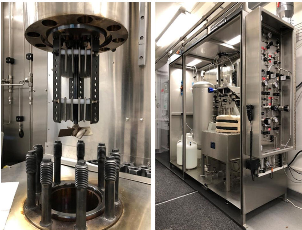
Figure 81 Design and setup of the high temperature and pressure corrosion testing facility at University of Iceland.
