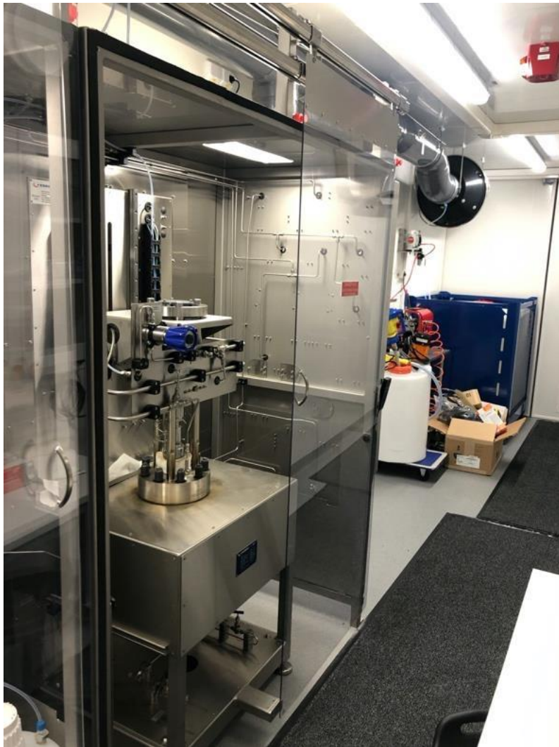
Figure 83 Autoclave setup used for simulating drilling environment.
