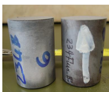
Coating adhesion failure
