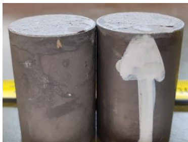
Coating cohesion failure
