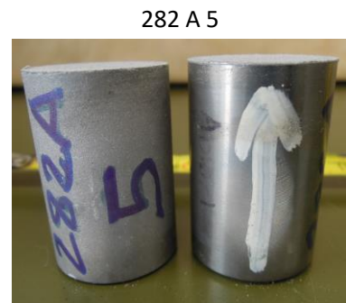
Dual failure mechanism due to both the adhesion of the coating and the failure of the glue
