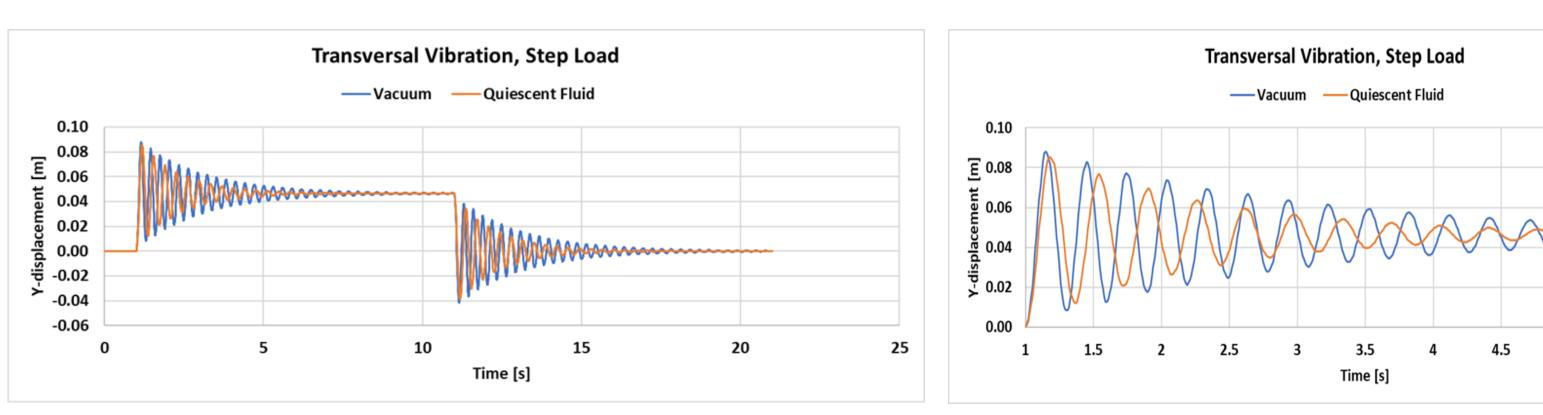
**Figure 9.** Structural dynamics of drill string, with added mass & added damping derived from CFD-FSI calculations
