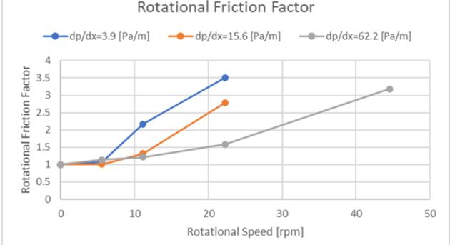
**Figure 8.** 3D CFD-LES results for annular flow with a rotating drill sting. Results are used to develop 1D models of rotating non-Newtonian fluids
