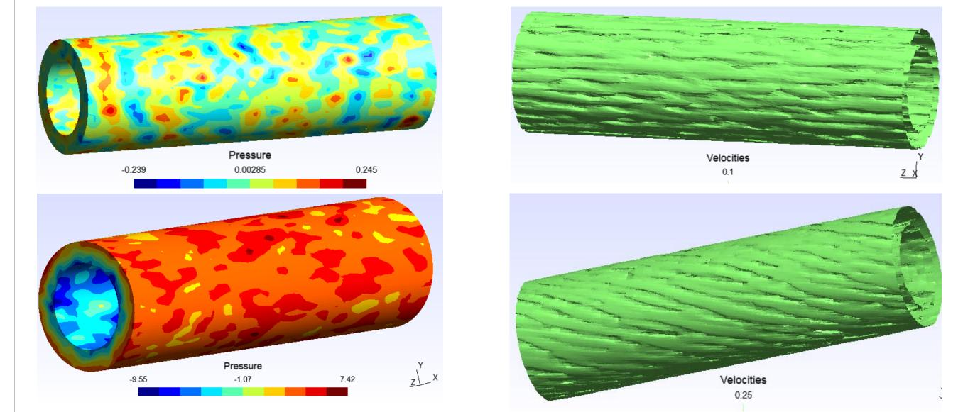
**Figure 3.** LES of annular flow: a) pressure fluctuations; b) velocity iso-surfaces. With rotating drill string: c) pressure fluctuations; d) velocity iso-surfaces
