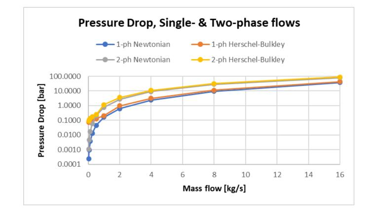
**Figure 6.** 1D flow assurance simulation results for single- and two-phase flows with Newtonian and non-Newtonian fluids (Herschel-Bulkley model)
