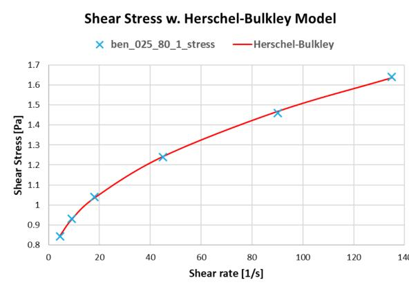
Figure 5. Herschel-Bulkley non-Newtonian fluid model tuned to rheological testing data. Implemented in both the 1D and 3D software.
