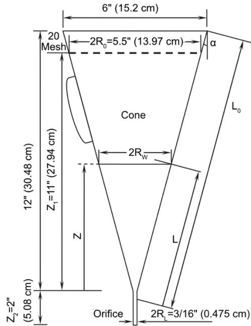
Figure 2. Schematic representation of standard Marsh-Funnel according to API 13B and DIN 4126.
