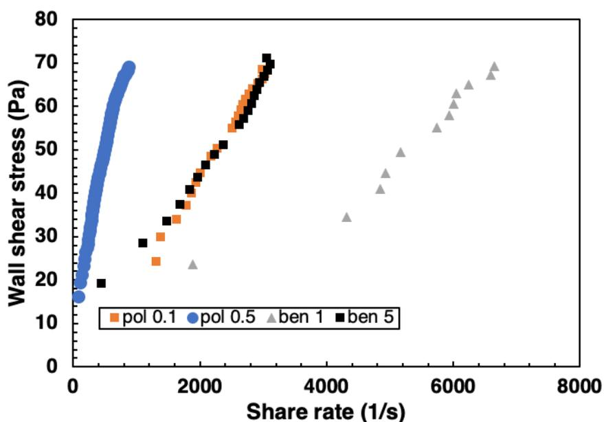
Figure 7. Shear stress as a function of shear rate for selected polymer and bentonite drilling muds determined from Marsh Funnel tests.
