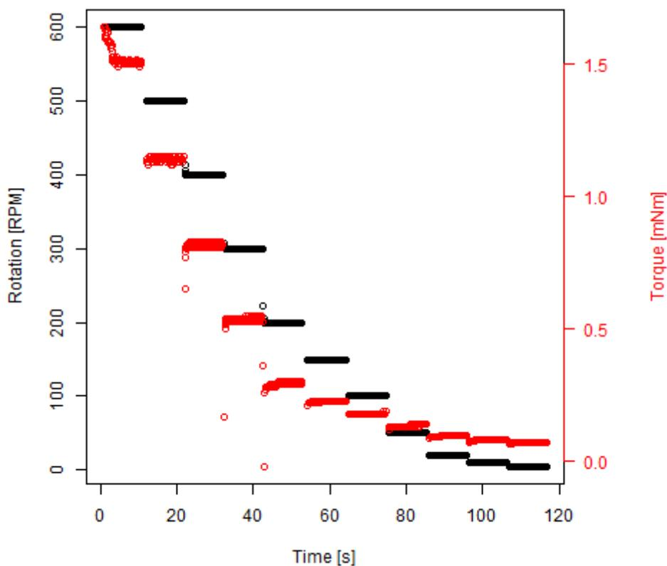
Figure 5. Angular velocity profile used by the HAAKE MARS Rheometer for this work. An example of measured torque is also displayed.
