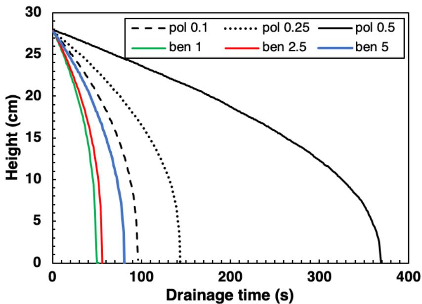
**Figure 6.** Drainage time for all drilling fluids tested with Marsh Funnel test as a function of fluid's height remaining in the funnel.
