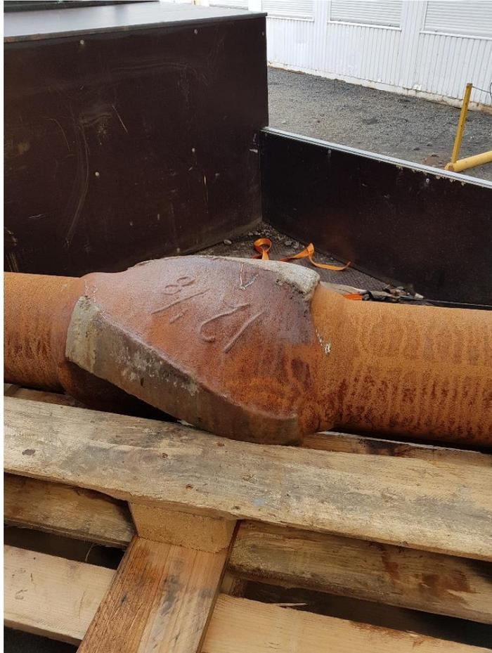
**Figure 7: worn down stabilizer blades<sup>††</sup>**
