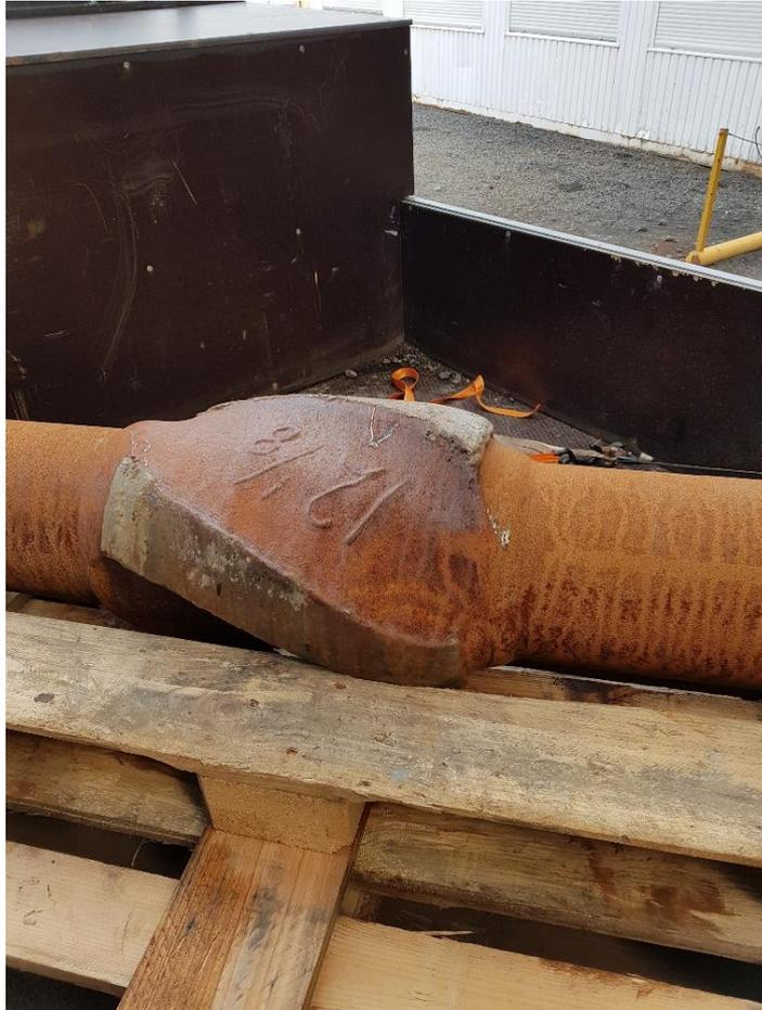
**Figure 7: worn down stabilizer blades<sup>††</sup>**
