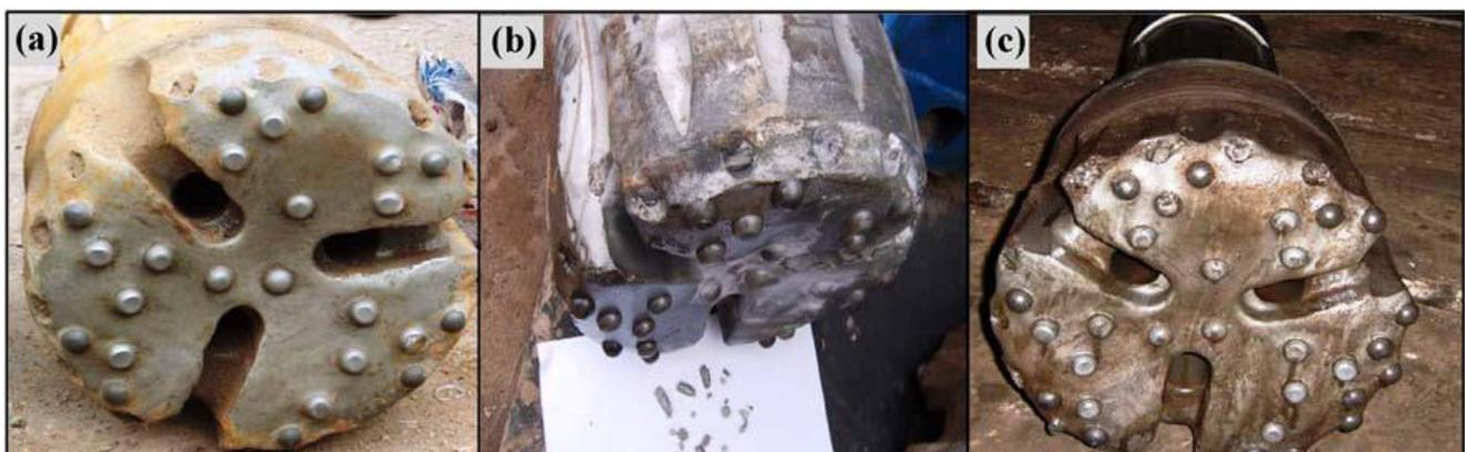
**Figure 4: Failure modes of the drill bits: (a) bit shank failure, (b) insert failure, and (c) insert wear †**
