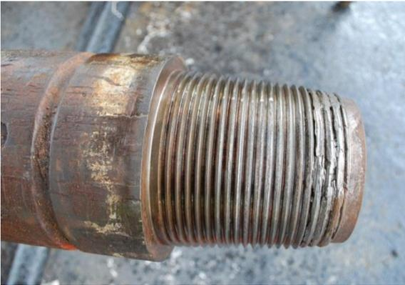
Figure 5: Thread galling<sup>§</sup>
