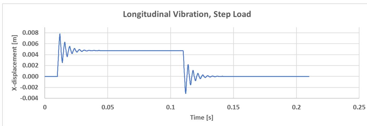
**Figure 3.1:** Results with the newly developed FEM structural dynamics solver using 20 finite elements. Time-history of free end of cantilever beam subjected to a longitudinal step load.
