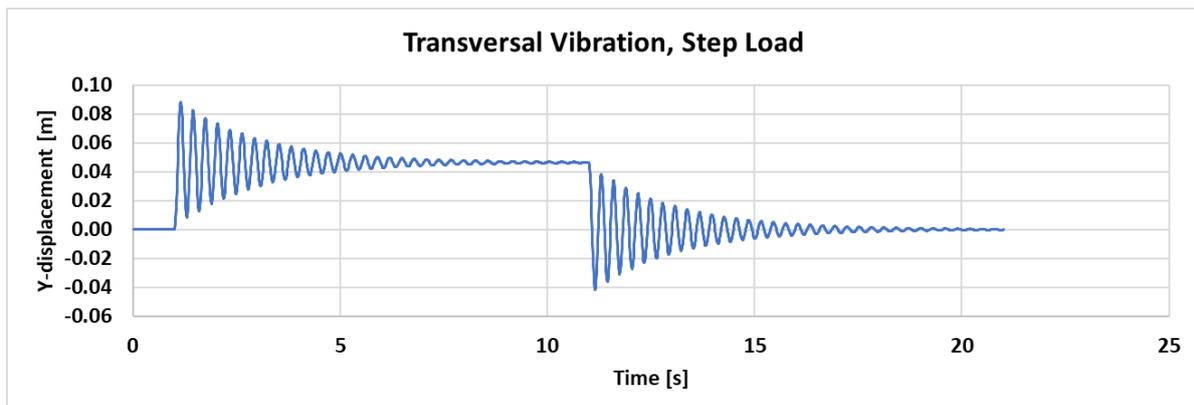
Figure 3.3: Results with the newly developed FEM structural dynamics solver using 20 finite elements. Time-history of free end of cantilever beam subjected to a transversal step load.
