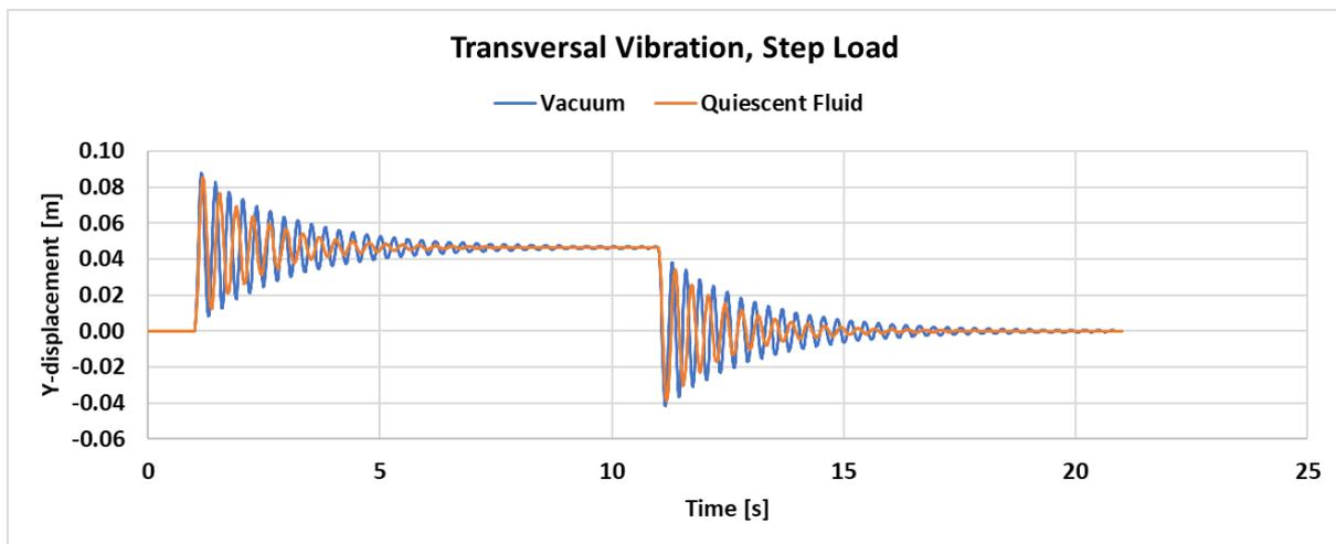
**Figure 4.1:** Time-history of free end of cantilever beam subjected to a transversal step load. Comparison of vibration in vacuum and in a quiescent fluid (=added mass and added damping included).
