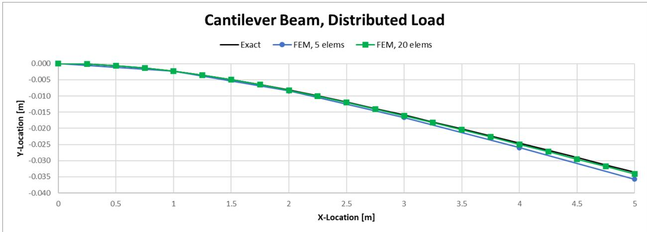
**Figure 2.1:** Results with the newly developed FEM solver using 5 and 20 finite elements, compared with the exact solution for slender beams. Notice that X- and Y-axes have different scales.
