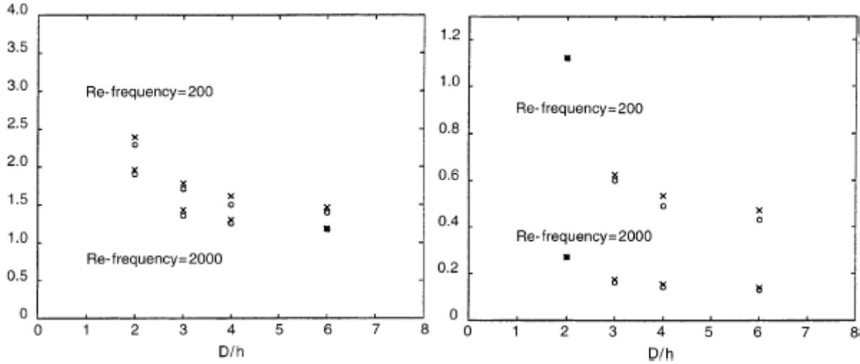
**Figure 4.5:** Normalized added mass ( $m_{ad}/(\frac{\rho\pi h^2}{4})$ ) and normalized added damping ( $c_{ad}/(\frac{\omega\rho\pi h^2}{4})$ ) versus D/h ratio for transversal vibrations of a circular cylinder in a quiescent fluid as calculated by Flowphys CFD [7] and by Chen [8]. a) Normalized added mass; b) Normalized added damping
