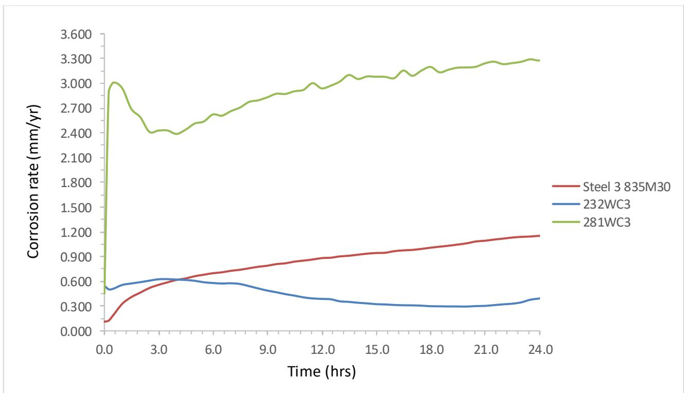
Figure 39 Corrosion rate for Coatings on Steel 3 after 24h testing in simulated drilling fluid
