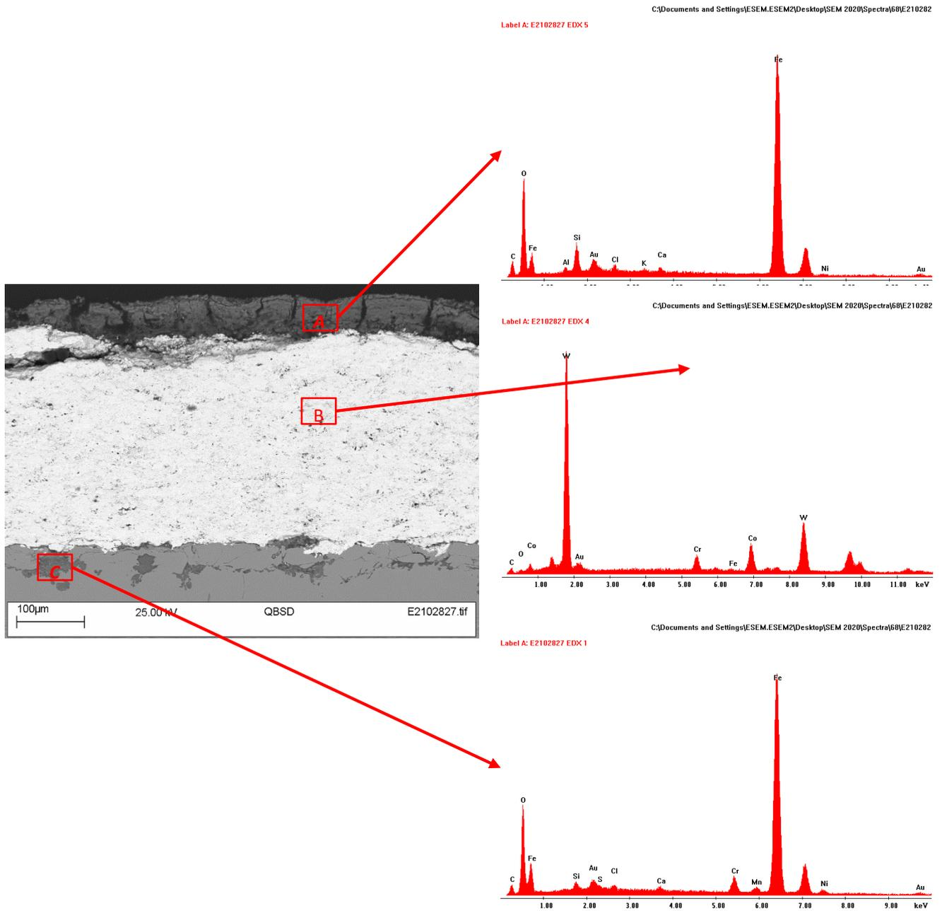
Figure 54 SEM and EDX analyse on polished cross-sectional surface of 232WC1 after 7-day testing
