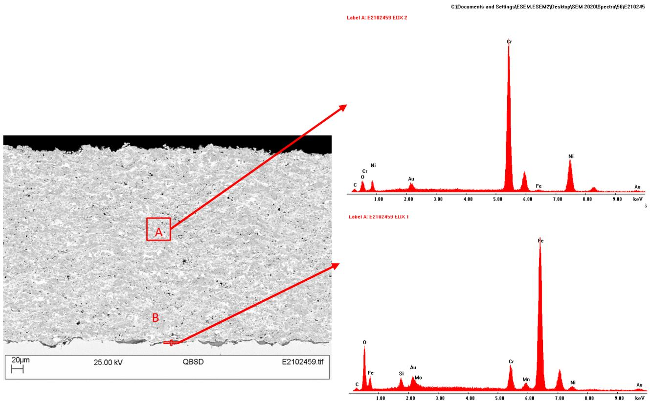
Figure 19 SEM and EDX analyse on polished cross-sectional surface of 233CrC1 after 24h testing
