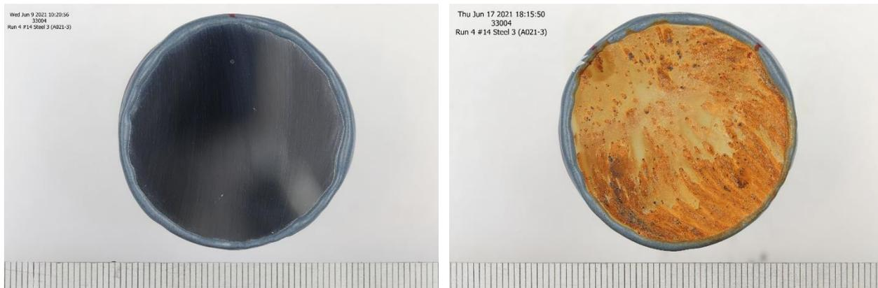
Figure 33 Digital images of Steel 3 after 24h testing: (left) before testing, (right) after testing
