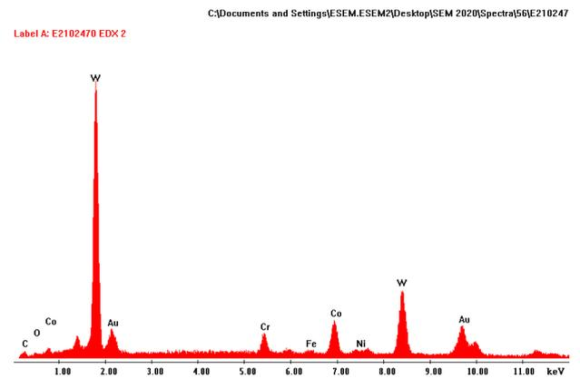
Figure 30 SEM and EDXanalyse on polished cross-sectional surface of 232WC2 after 24h testing
