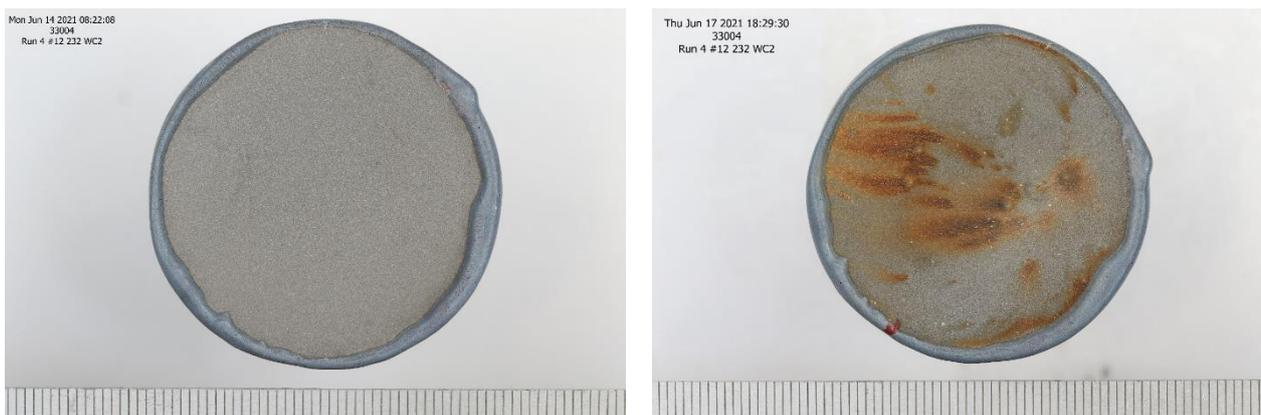
Figure 27 Digital images of 232WC2 after 24h testing: (left) before testing, (right) after testing
