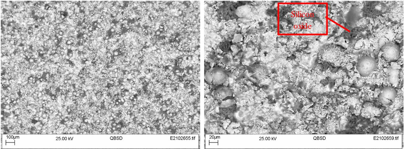
Figure 49 SEM and EDX analyse on top surface of 234Flux1 after 7-day testing
