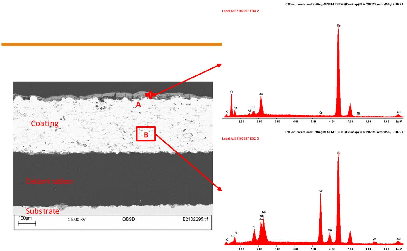
Figure 21 SEM and EDX analyse on polished cross-sectional surface of 235Amor1 after 24h testing
