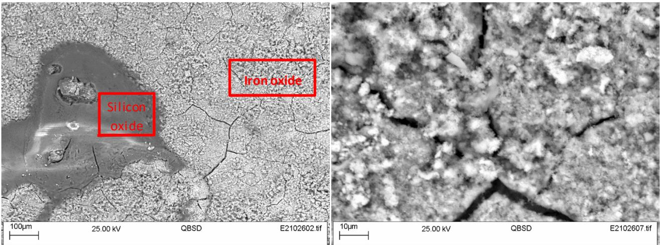
Figure 46 SEM and EDX analyse on top surface of Steel 1 after 7-day testing
