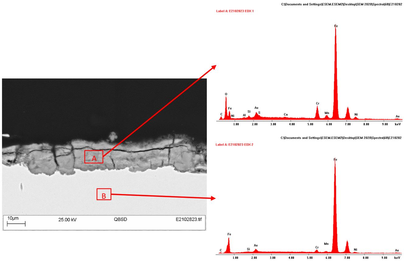
Figure 52 SEM and EDX analyse on polished cross-sectional surface of Steel 1 after 7-day testing
