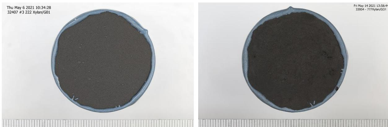
Figure 7 Digital images of 222Xylan/GO after 24h testing: (left) before testing, (right) after testing
