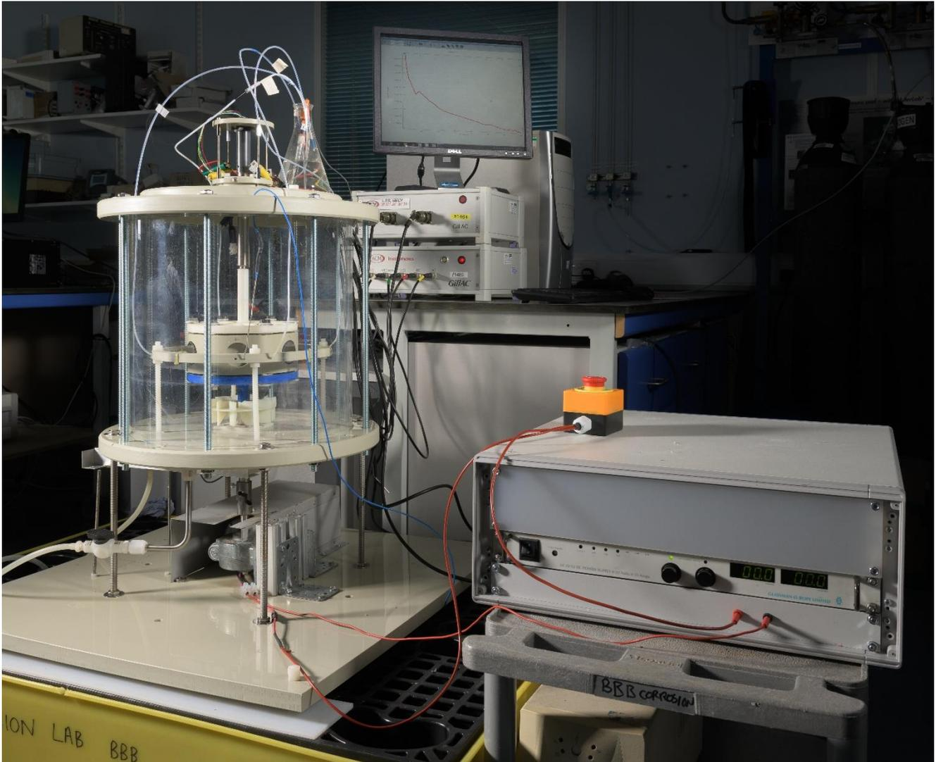
Figure 3 A photograph of TWI's erosion-corrosion facility
