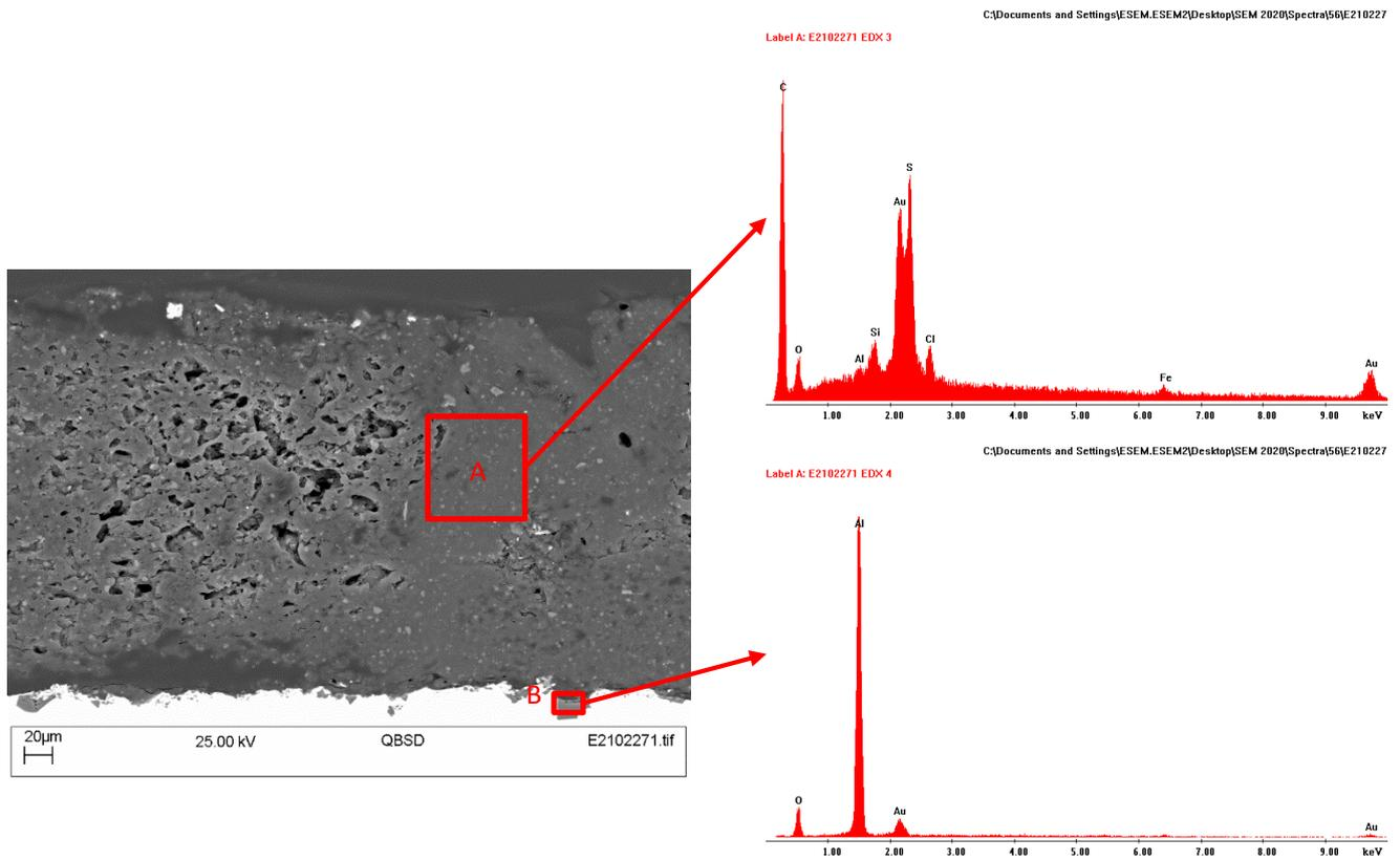
Figure 17 SEM and EDX analyse on polished cross-sectional surface of 222Xylan/GO after 24h testing
