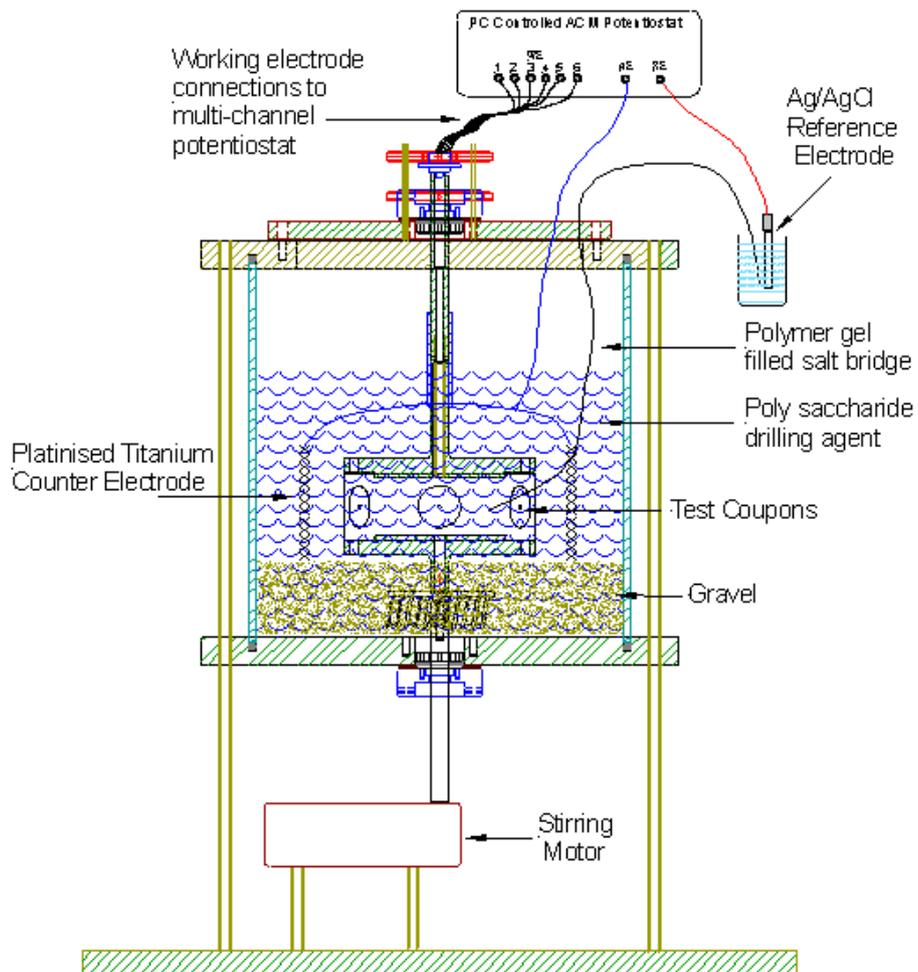
Figure 2 The design of TWI's erosion-corrosion facility
