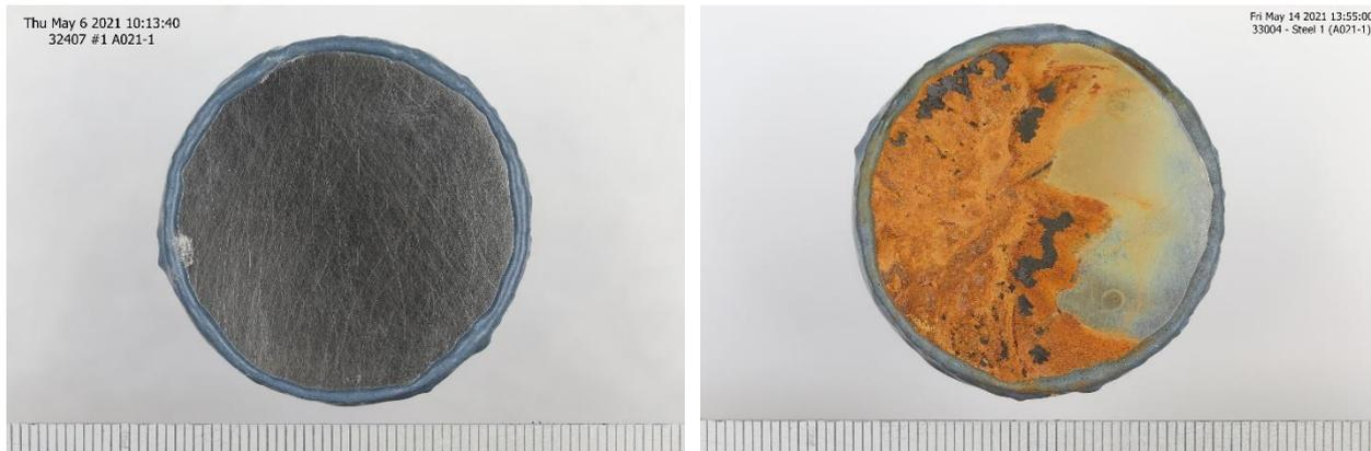
Figure 5 Digital images of Steel 1 after 24h testing: (left) before testing, (right) after testing
