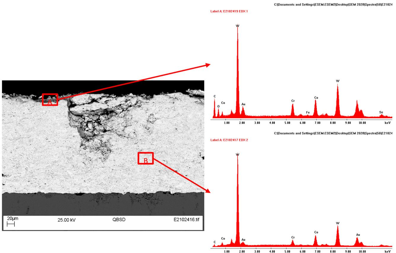
Figure 37 SEM and EDXanalyse on polished cross-sectional surface of 232WC3 after 24h testing
