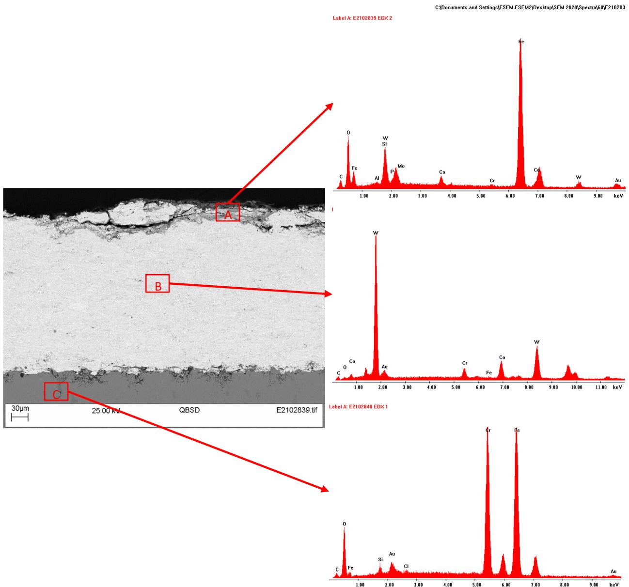
Figure 57 SEM and EDX analyse on polished cross-sectional surface of 232WC2 after 7-day testing
