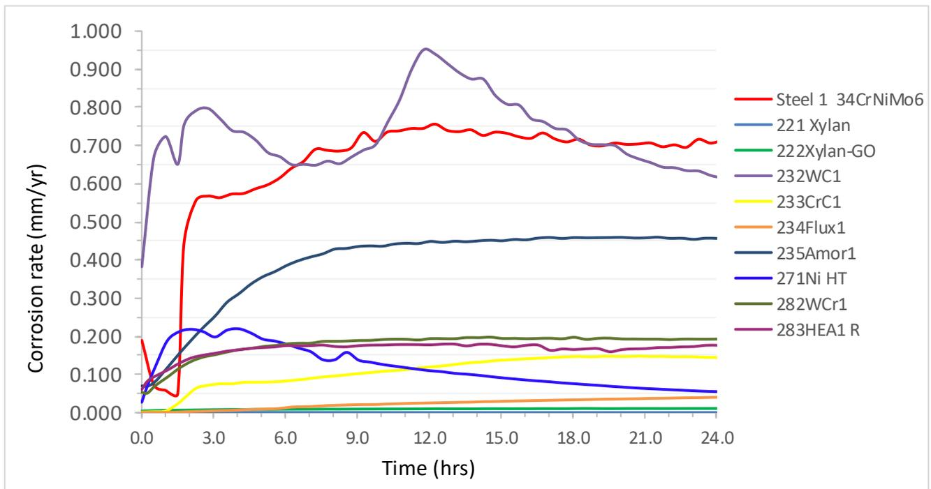
Figure 25 Corrosion rate for Coatings on Steel 1 after 24h testing in simulated drilling fluid
