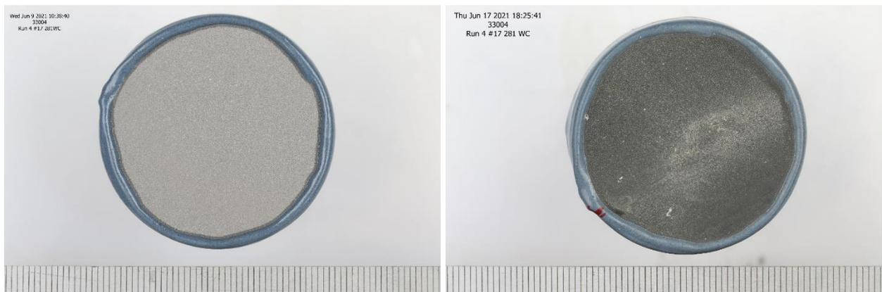
Figure 35 Digital images of 281WC3 after 24h testing: (left) before testing, (right) after testing
