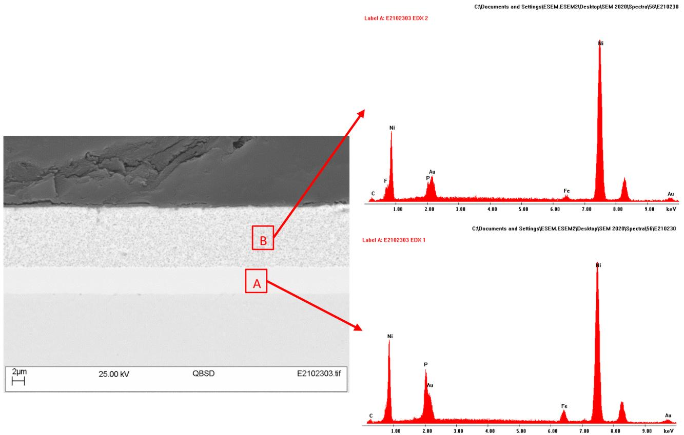
Figure 22 SEM and EDX analyse on polished cross-sectional surface of 271Ni after 24h testing
