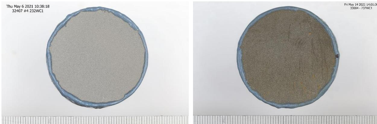
Figure 8 Digital images of 232WC1 after 24h testing: (left) before testing, (right) after testing
