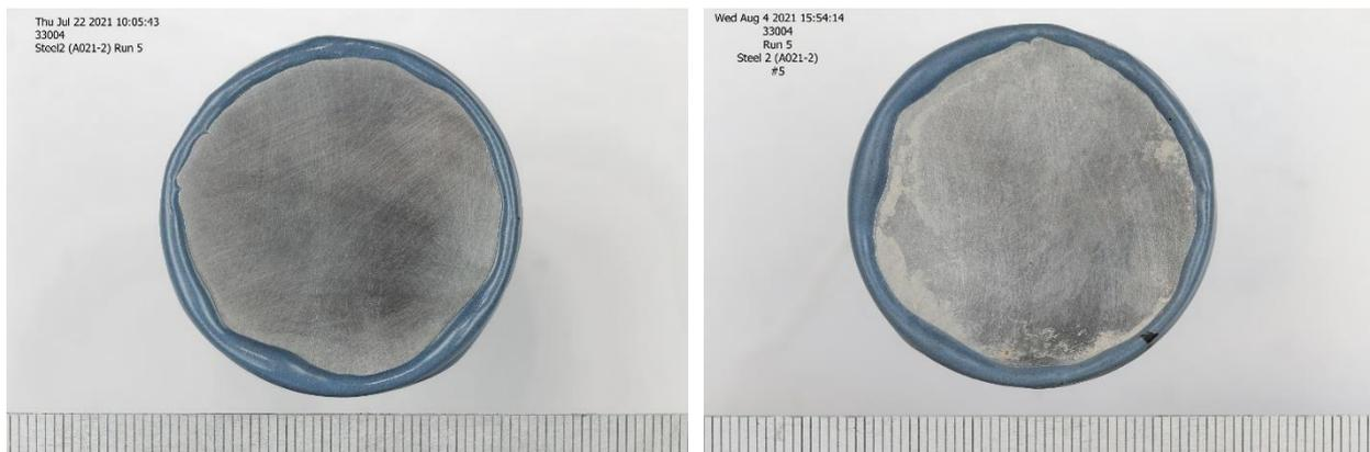
Figure 44 Digital images of Steel 2 after 7-day testing: (left) before testing, (right) after testing
