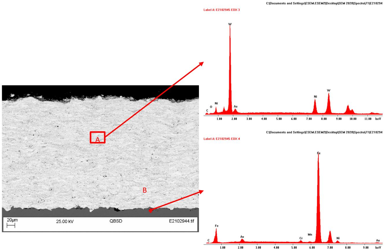
Figure 38 SEM and EDXanalyse on polished cross-sectional surface of 281WC3 after 24h testing
