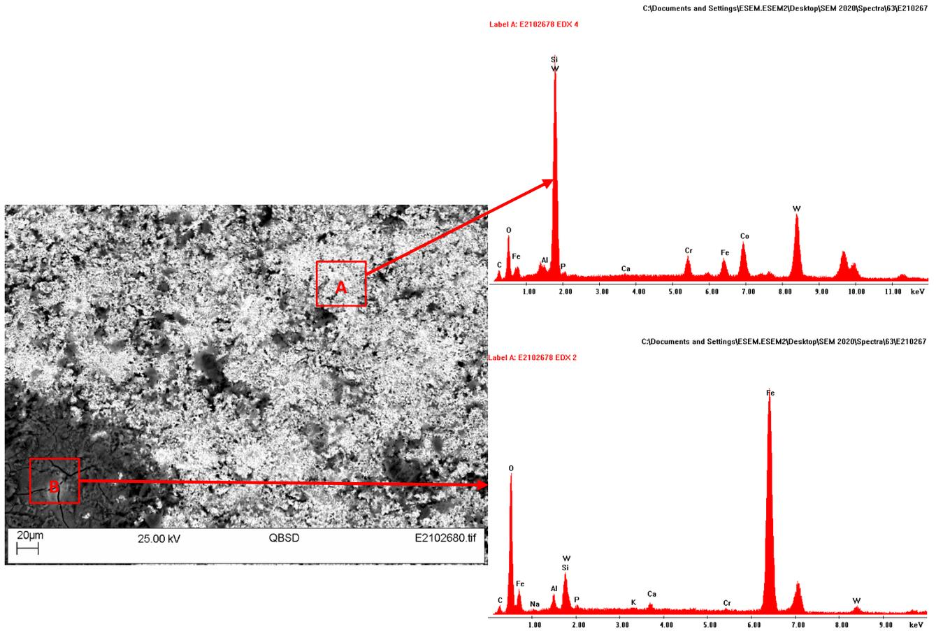
Figure 51 SEM and EDX analyse on top surface of 232WC2 after 7-day testing
