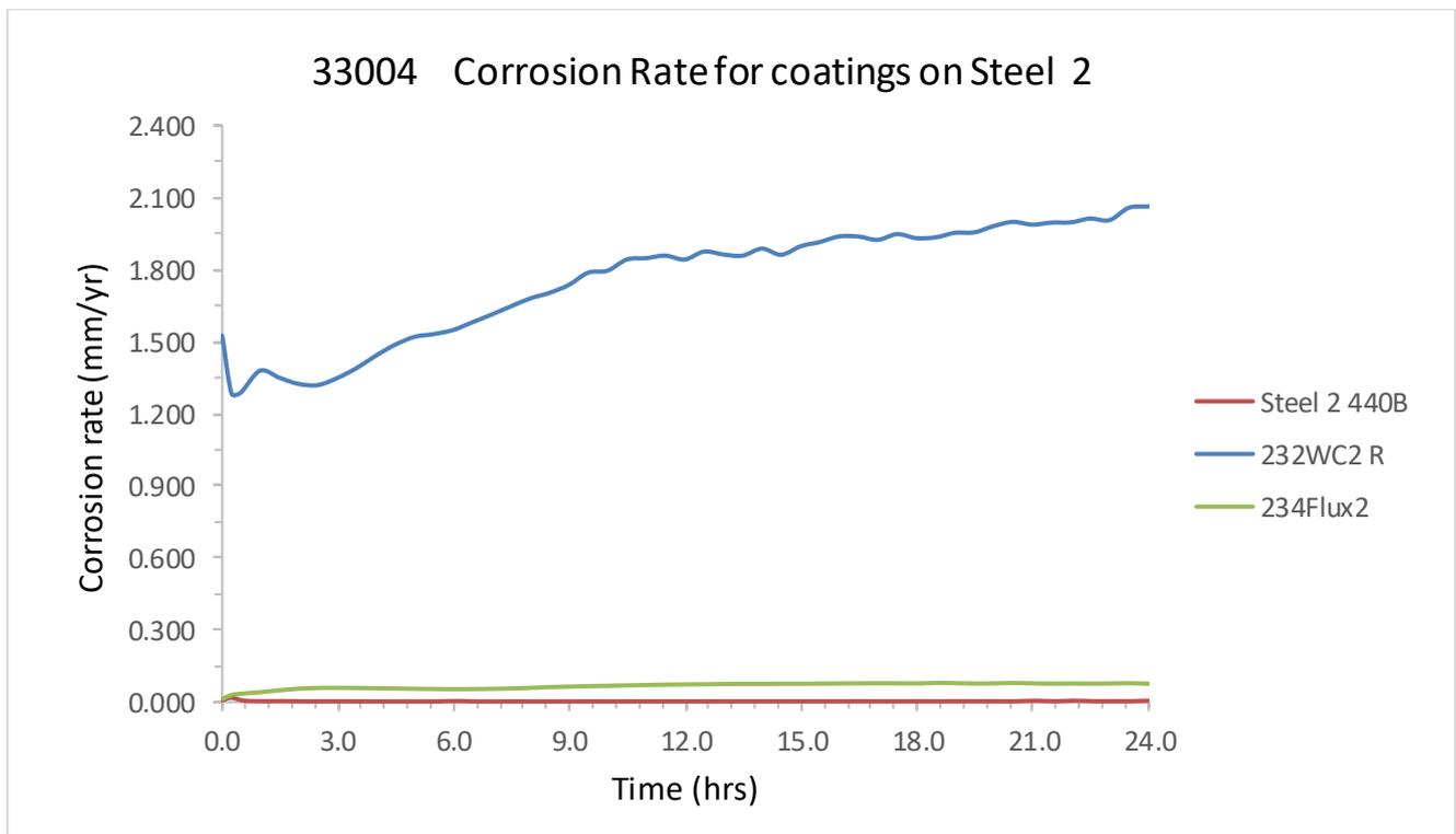
Figure 32 Corrosion rate for Coatings on Steel 2 after 24h testing in simulated drilling fluid
