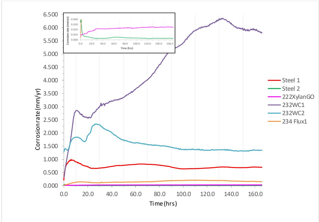
Figure 58 Corrosion rate for Coatings on Steel 3 after 24h testing in simulated drilling fluid
