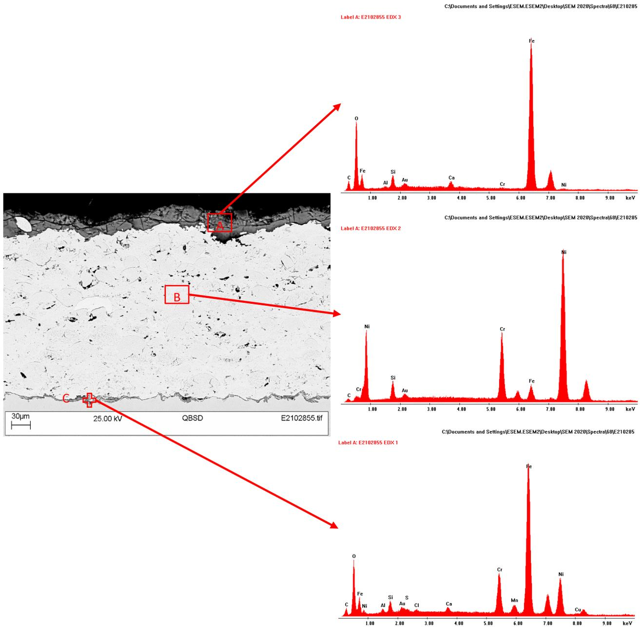
Figure 55 SEM and EDX analyse on polished cross-sectional surface of 234Flux1 after 7-day testing
