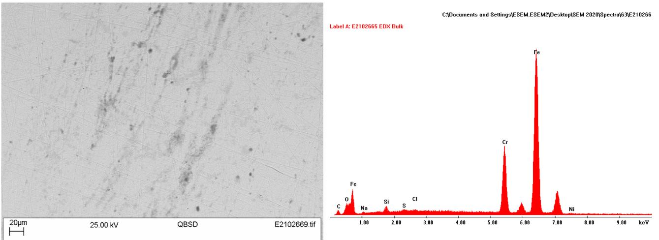
Figure 50 SEM and EDX analyse on top surface of Steel 2 after 7-day testing
