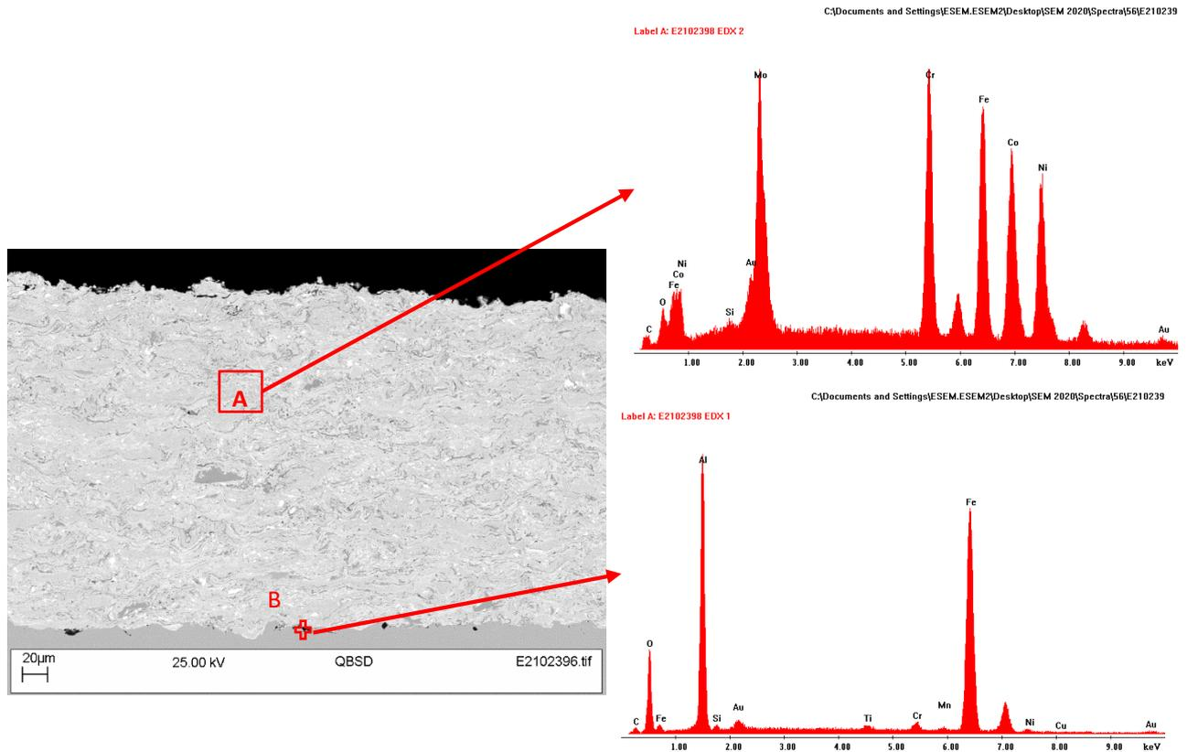
Figure 24 SEM and EDX analyse on polished cross-sectional surface of 283HEA1 after 24h testing **R**
