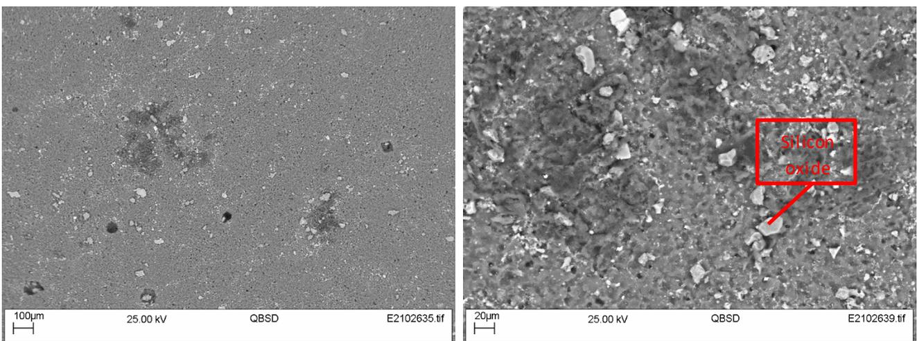
Figure 47 SEM and EDX analyse on top surface of 222Xylan/GO1 after 7-day testing
