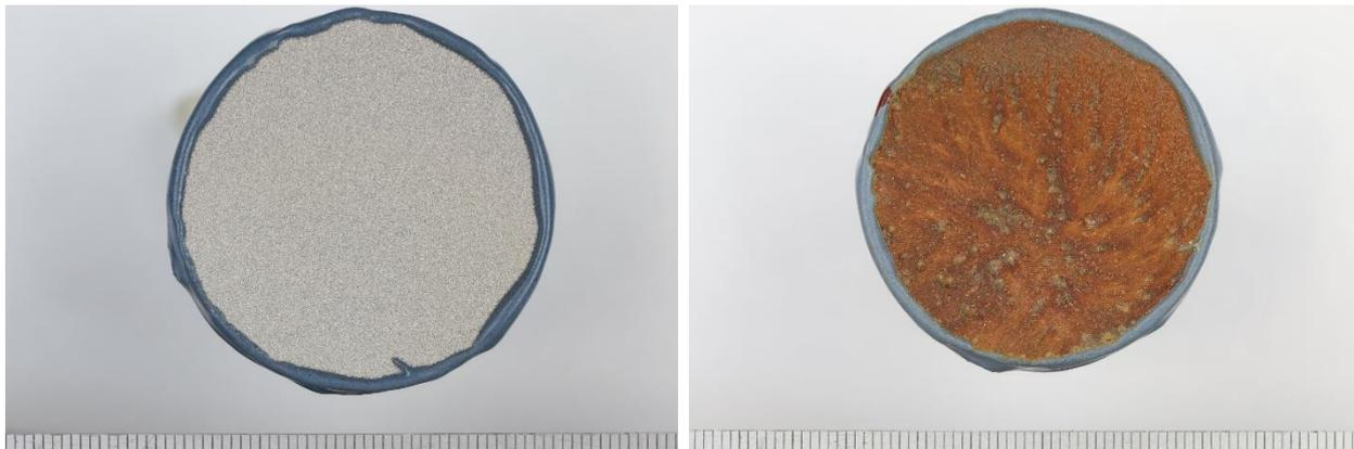
Figure 11 Digital images of 235Amor1 after 24h testing: (left) before testing, (right) after testing
