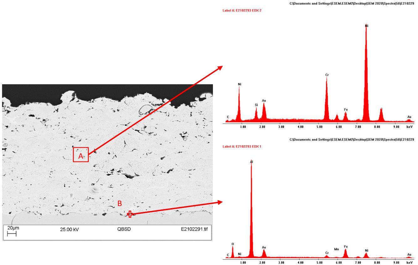
Figure 20 SEM and EDX analyse on polished cross-sectional surface of 234Flux1 after 24h testing
