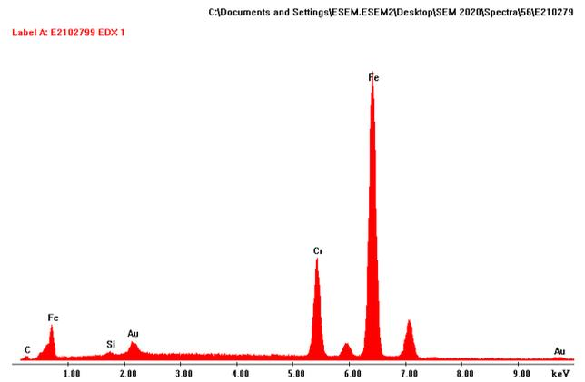
Figure 29 SEM and EDXanalyse on polished cross-sectional surface of Steel 2 after 24h testing
