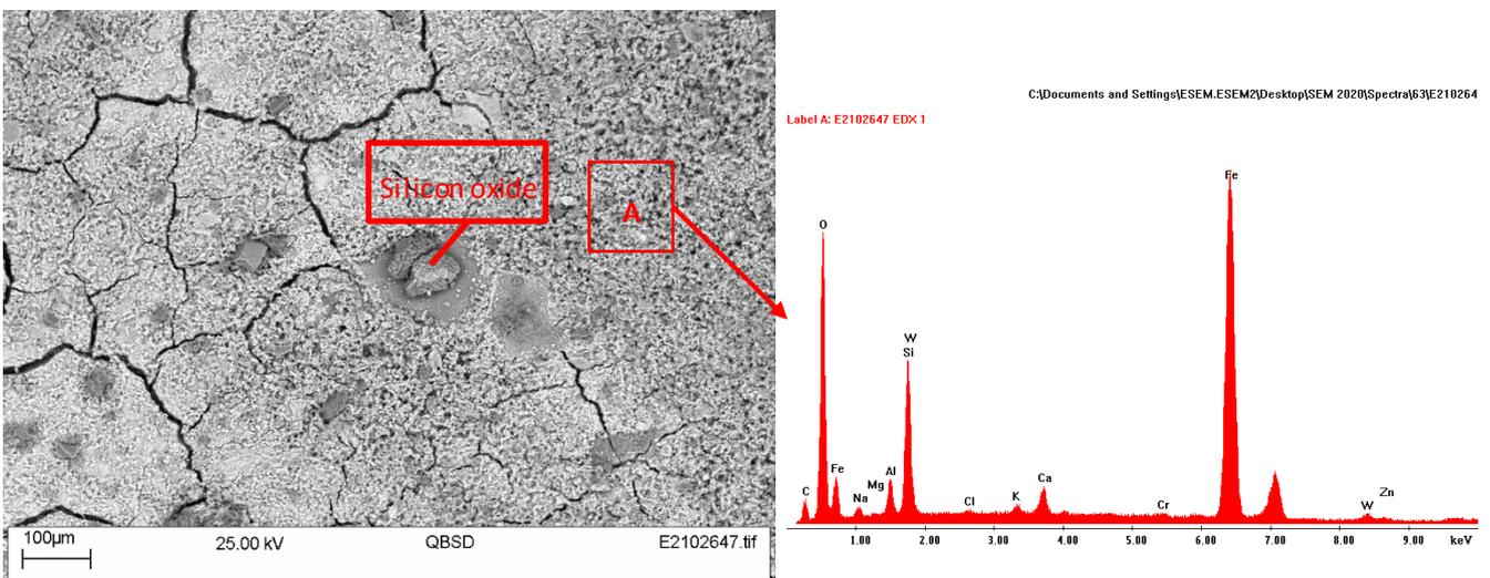
Figure 48 SEM and EDX analyse on top surface of 232WC1 after 7-day testing
