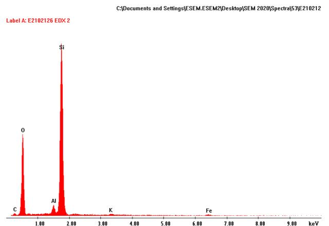
Figure 4 SEM and EDX analyse of sand particles added into simulated drilling fluid
