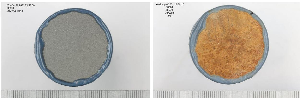
Figure 42 Digital images of 232WC1 after 7-day testing: (left) before testing, (right) after testing
