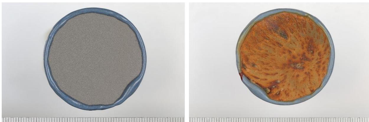
Figure 13 Digital images of 282WCr1 after 24h testing: (left) before testing, (right) after testing
