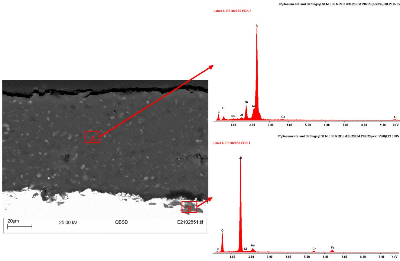
Figure 53 SEM and EDX analyse on polished cross-sectional surface of 222Xylan/GO1 after 7-day testing
