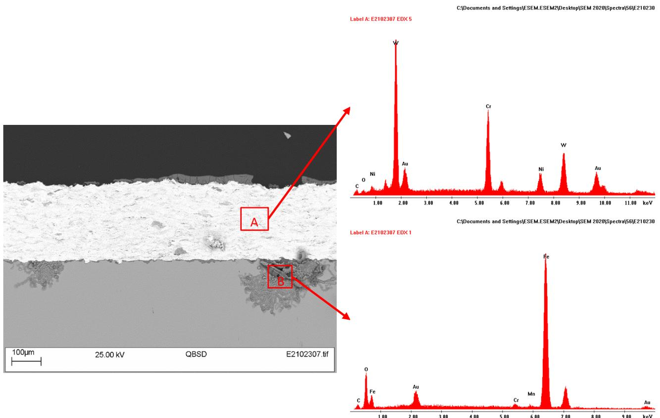
Figure 23 SEM and EDX analyse on polished cross-sectional surface of 282WCr1 after 24h testing
