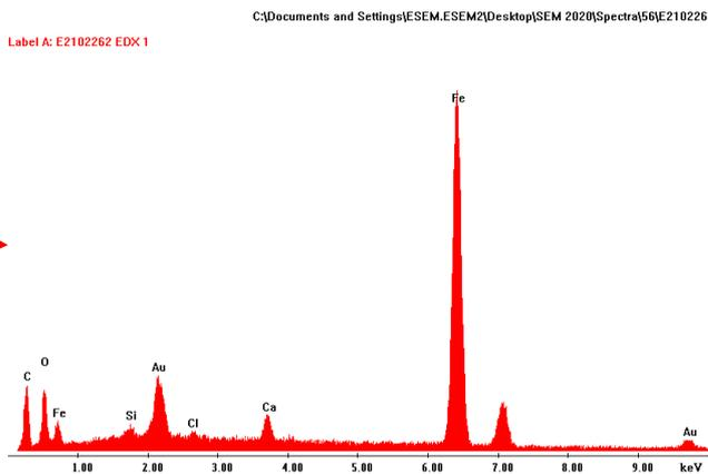
Figure 15 SEM and EDX analyse on polished cross-sectional surface of Steel 1 after 24h testing
