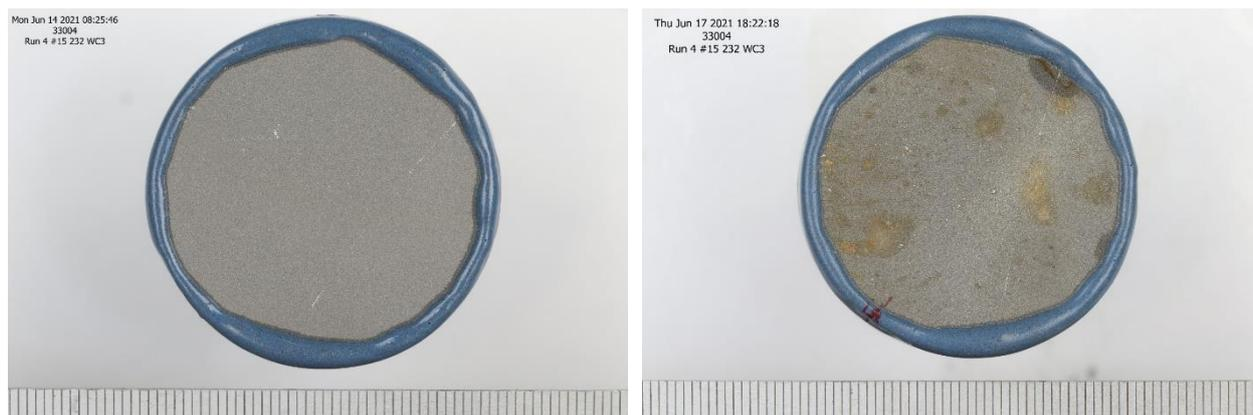
Figure 34 Digital images of 232WC3 after 24h testing: (left) before testing, (right) after testing
