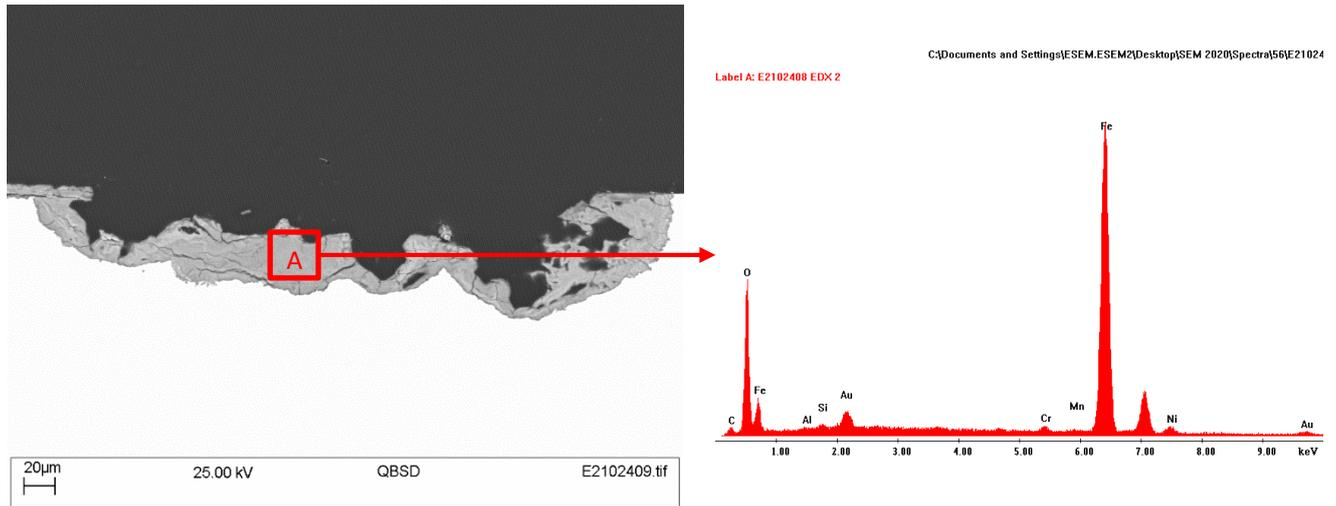
Figure 36 SEM and EDX analyse on polished cross-sectional surface of Steel 3 after 24h testing
