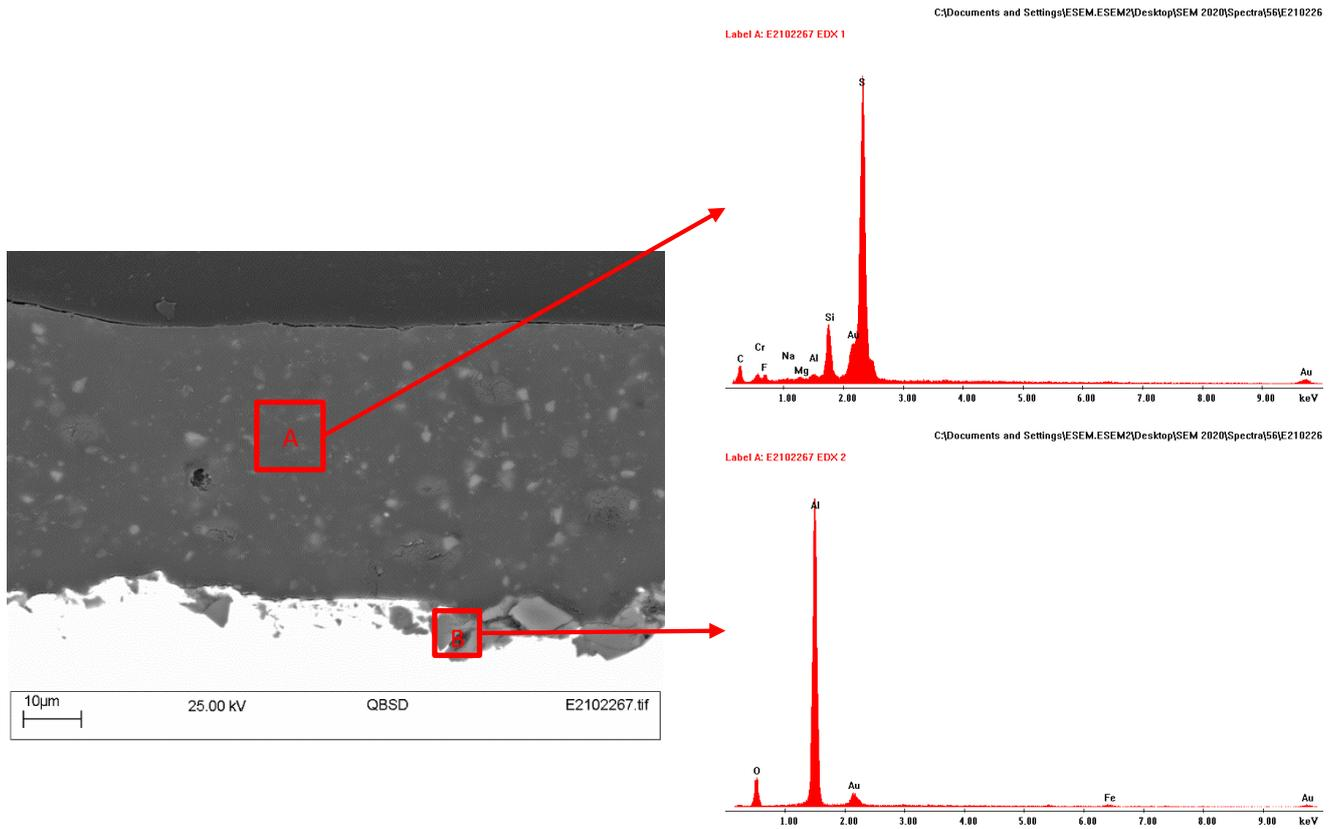
Figure 16 SEM and EDX analyse on polished cross-sectional surface of 221Xylan after 24h testing
