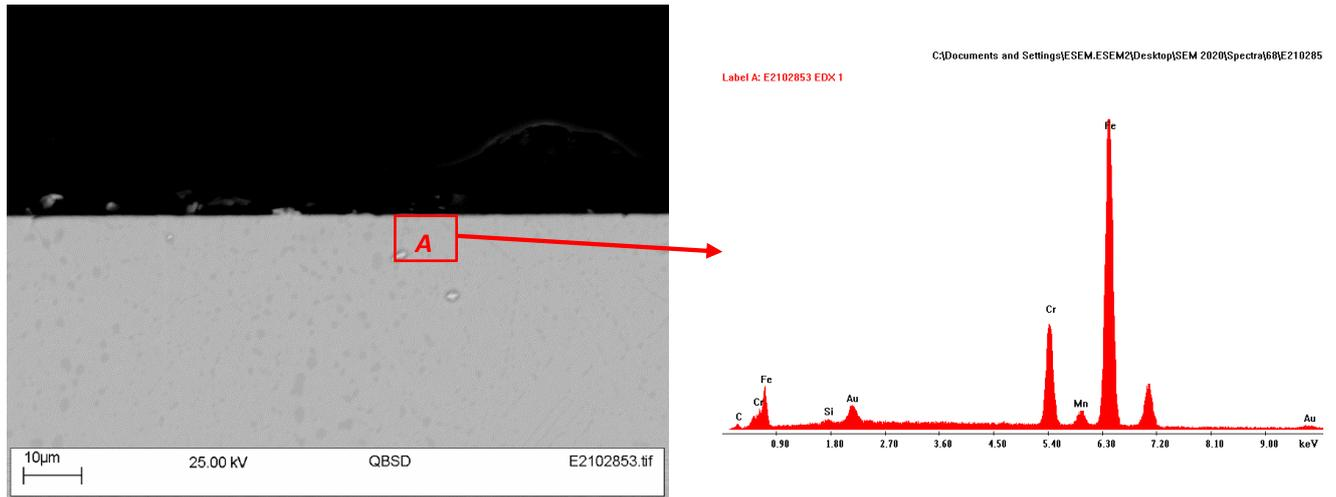
Figure 56 SEM and EDX analyse on polished cross-sectional surface of Steel 2 after 7-day testing
