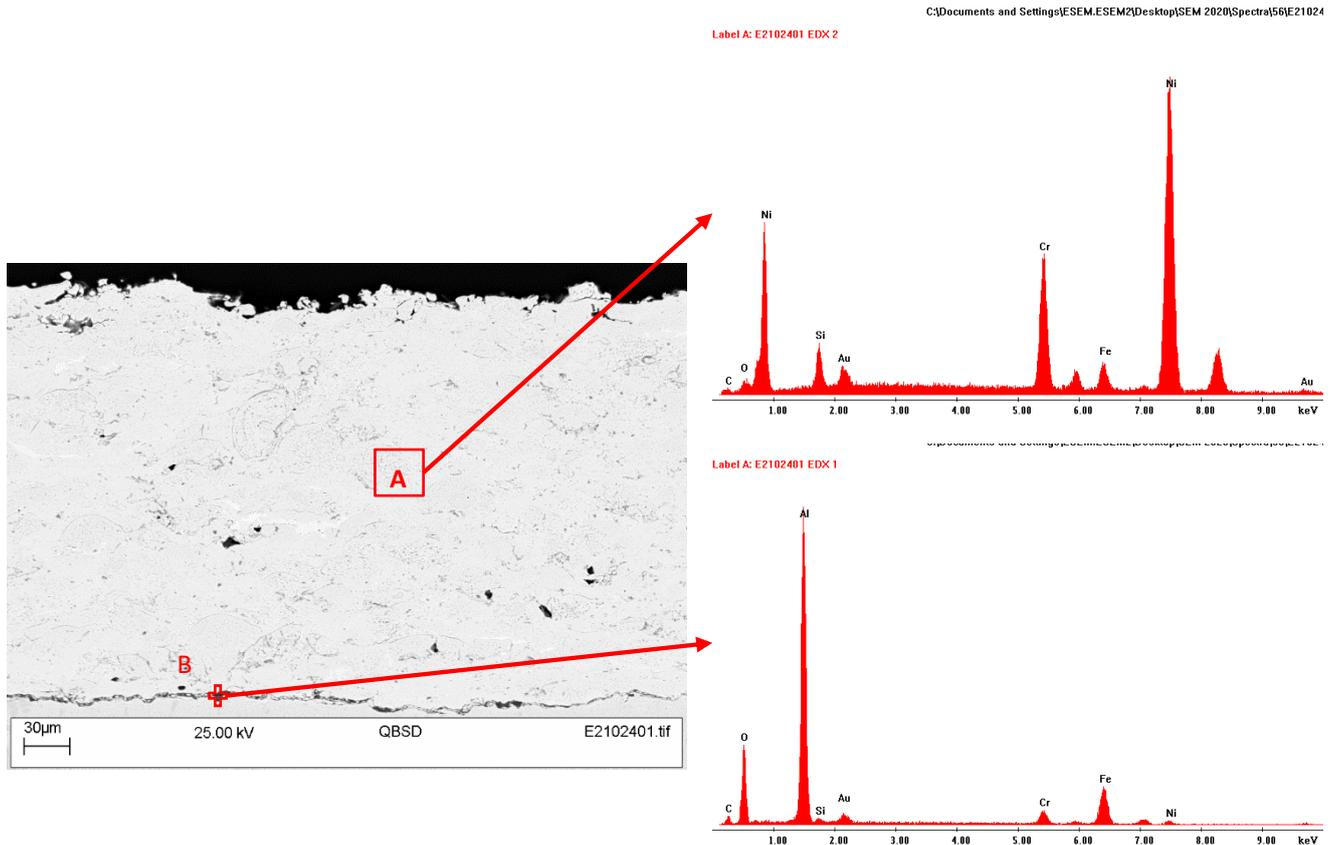
Figure 31 SEM and EDX analyse on polished cross-sectional surface of 234Flux2 after 24h testing
