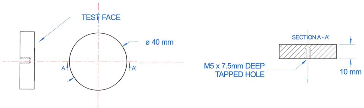
Figure 1 Design of test coupon for Geo-Drill erosion-corrosion testing
