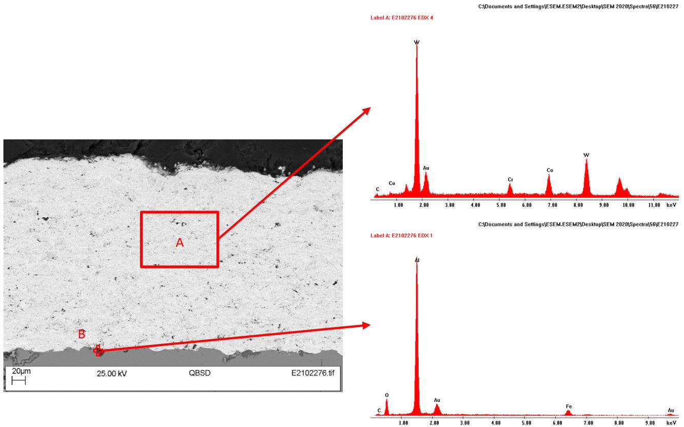
Figure 18 SEM and EDX analyse on polished cross-sectional surface of 232WC1 after 24h testing
