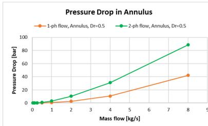
Figure 7. 1D flow assurance simulation results for annular flow single- and two-phase flows
