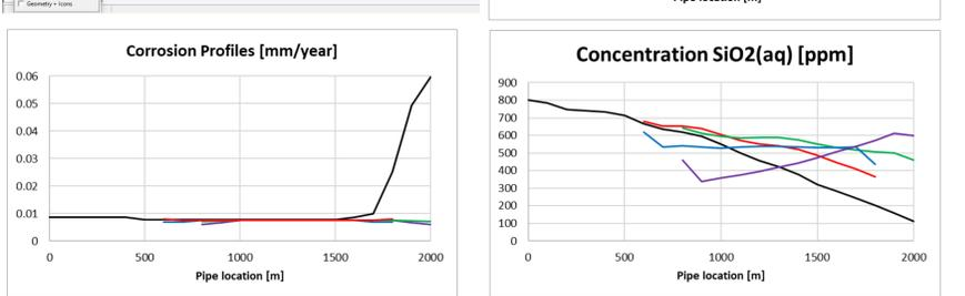
Figure 4. Geothermal Flow Assurance software: a) GUI showing a network model; b)-d) Simulation results for pressure, corrosion rate, concentrations. In addition, flow rate, temperature, density, volume/mass fractions, saturation indices, erosion rates, scaling rates are also available
