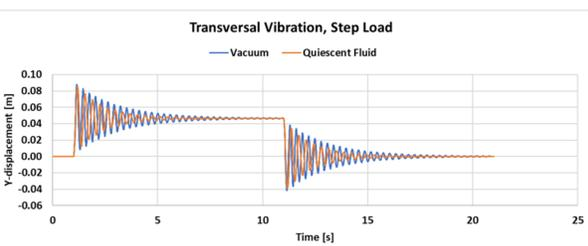
Figure 9. Structural dynamics of drill string, with added mass & added damping derived from CFD-FSI calculations
