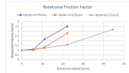
Figure 8. 3D CFD-LES results for annular flow with a rotating drill string. Results are used to develop 1D models of rotating non-Newtonian fluids
