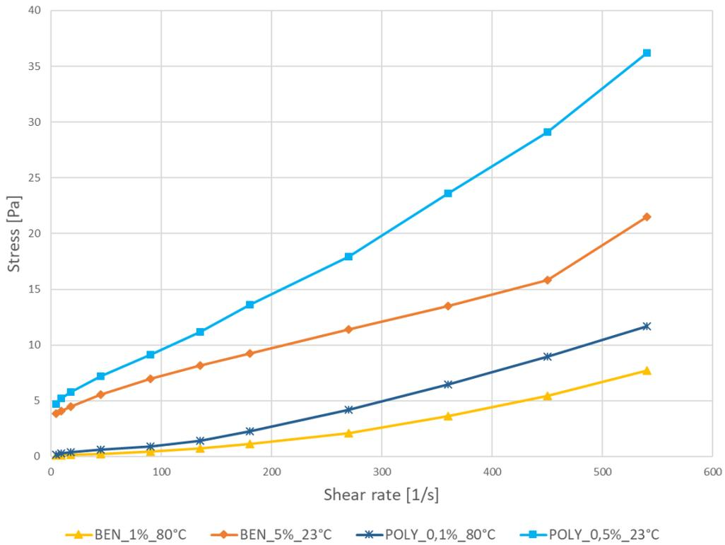
Figure 10. Shear stress as a function of shear rate for two polymer and two bentonite drilling muds measured with the HAAKE MARS rheometer.
