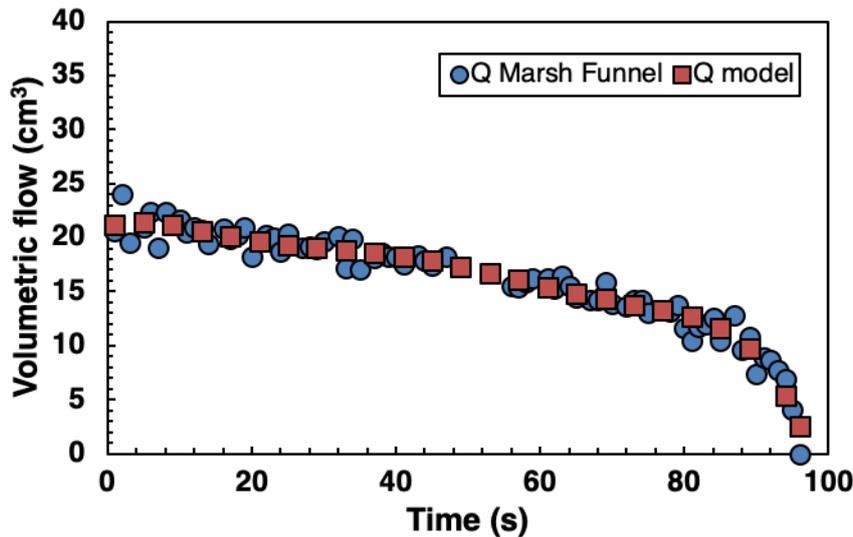
**Figure 3.** Measured flow rate of spilling drilling fluid (0.1 wt.% polymer based) and Herschel-Bulkley model fit.
