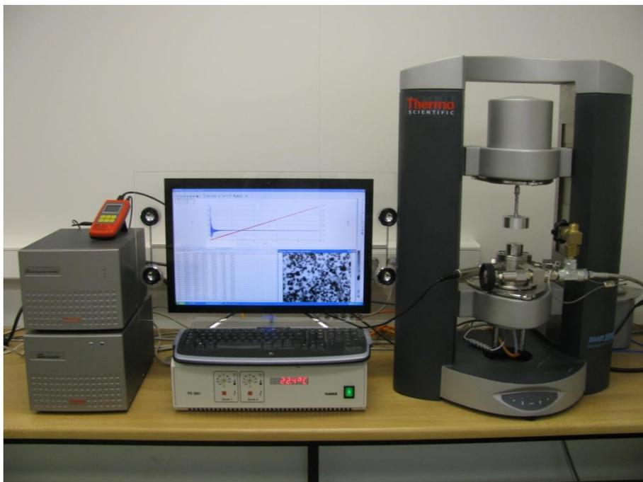
Figure 4. The HAAKE MARS (Rheomicroscope) used in this study.
