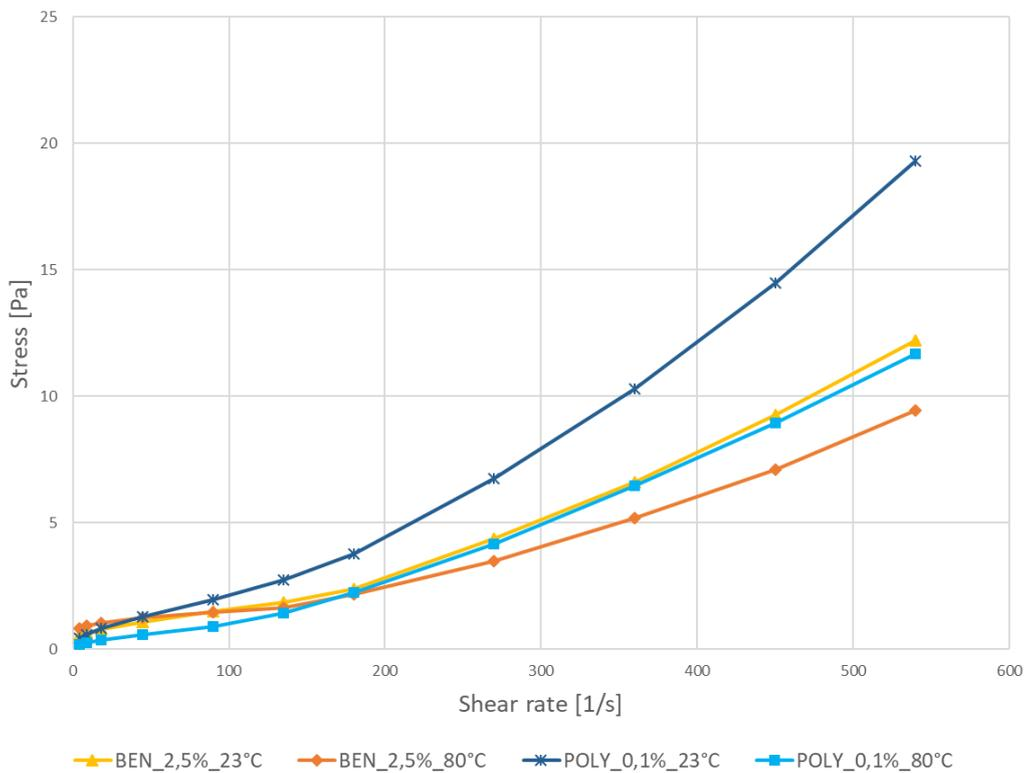
Figure 11. Shear stress as a function of shear rate for polymer and bentonite drilling muds as recommended by the supplier measured with the HAAKE MARS rheometer.
