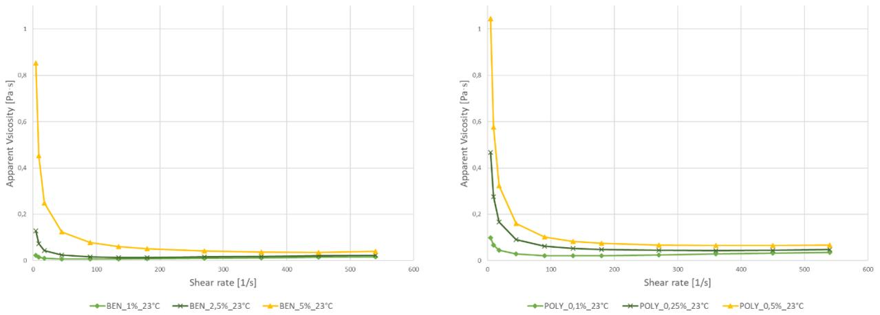
Figure 13. Apparent viscosity as a function of shear rate for bentonite and polymer drilling muds at 23°C measured with the HAAKE MARS rheometer.
