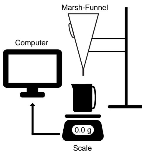
Figure 1. Arrangement of the equipment using a scale with automated data logging.
